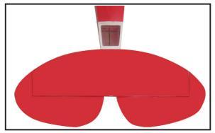
$\Box$  4) With the stabilizer held firmly in place, use a pen and draw lines onto the stabilizer where it and the fuselage sides meet. Do this on both the right and left sides and top and bottom of the stabilizer.
