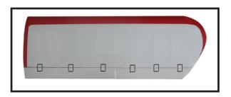
Note: Work the aileron up and down several times to "work in" the hinges and check for proper movement.
