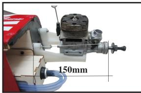
2) Use a pin drill and 4mm drill bit to drill a small indentation in the mount for the engine mounting screw.
