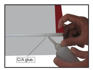
$\Box$  5) Turn the wing panel over and deflect the flap in the opposite direction from the opposite side. Apply thin C/A glue to each hinge, making sure that the C/A penetrates into both the flap and wing panel.
