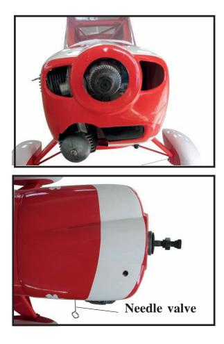
□ 3) Install the muffler and muffler extension onto the engine and make the cutout in the cowl for muffler clearance. Connect the fuel and pressure lines to the carburetor, muffler and fuel filler valve. Secure the cowl to fuselage using the M3x10mm screws.
