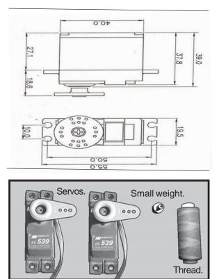
Because the size of servos differ, you may need to adjust the size of the precut opening in the mount. The notch in the sides of the mount allow the servo lead to pass through.
