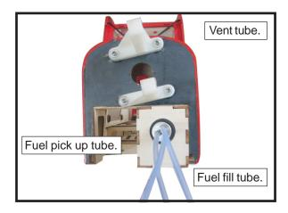
9) Connect the lines from the tank to the engine and muffler. The vent line will connect to the muffler and the line from the clunk to the carburetor.
