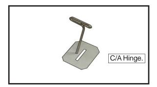
□ 2) Remove each hinge from the wing panel and flap and place a T-pin in the center of each hinge. Slide each hinge into the aileron until the T-pin is snug against the aileron. This will help ensure an equal amount of hinge is on either side of the hinge line when the flap is mounted to the wing panel.
