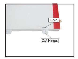
$\Box$  3) Slide the flap on the wing panel until there is only a slight gap. The hinge is now centered on the wing panel and flap. Remove the T-pins and snug the flap against the wing panel. A gap of 1/64" or less should be maintained between the wing panel and flap.
