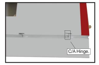
□ 4)Deflect the flap and completely saturate each hinge with thin C/A glue. The ailerons front surface should lightly contact the wing during this procedure. Ideally, when the
