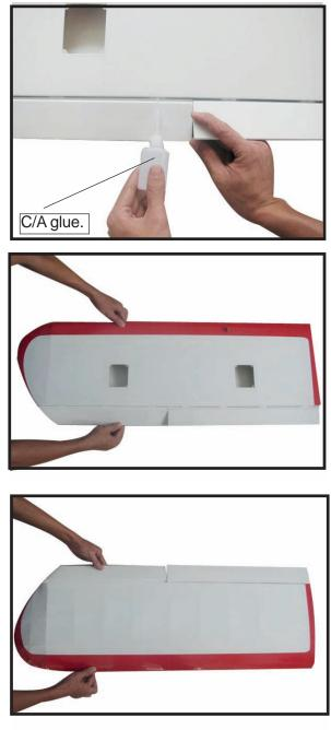
□ 5) Turn the wing panel over and deflect the aileron in the opposite direction from the opposite side. Apply thin C/A glue to each hinge, making sure that the C/A penetrates into both the aileron and wing panel.
