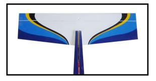
10) After the epoxy has fully cured, remove the masking tape or T-pins used to hold the stabilizer in place. Carefully inspect the glue joints. Use more epoxy to fill in any gaps that may exist that were not filled previously and clean up the excess using a paper towel and rubbing alcohol.
