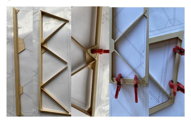
5) Stick the horizontal tail fin according to the drawing position.
