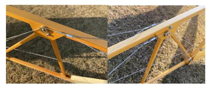
12) Installation of the bracing wires for the fuselage and tail.
