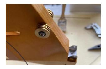
5) Install landing skid connections with tapping screws.
