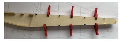
11) Joint 12X16MM pine strips according to the drawing, and strengthen the top position with pine.
