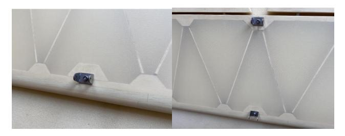
2) Assemble the tail fins on the fuselage, mark the position where need to drill a 3MM hole, keeping the perpendicularity of the holes.
