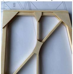
5) Stick 5X16MM pine strips up and down the fuselage.
