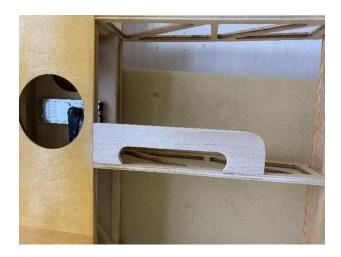
21) Assemble ailerons according to the rib numbers and paste reinforcement plates.
