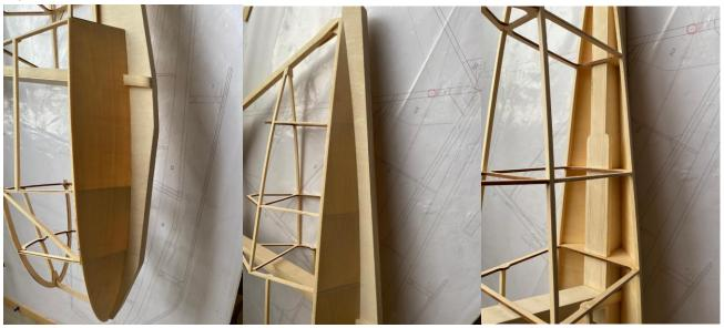
25) Stick the balsa sheets and polish to be radian, so that the cover has a larger bonding area.
