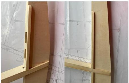
20) Assemble and stick the two pcs of A3 polywood sheets and build the cockpit according to the position in the drawing.
