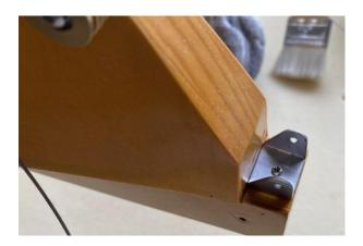
4) Install pulley with M3 screws.
