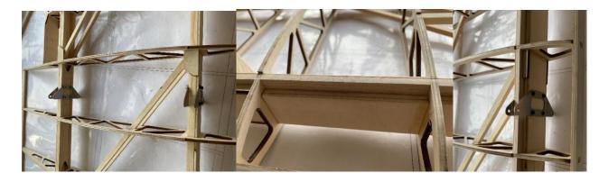
15) Wing tip sticked balsa wood can be increased the pasting area.
