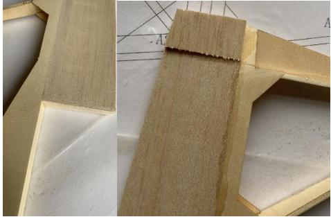
3) The position of horns should be reinforced with pine blocks.
