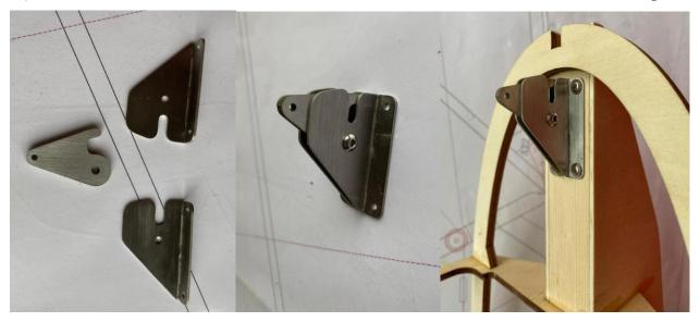
22) The tow hook is needed to be bent, assembled with 3MM screws and mounted to the fuselage.
