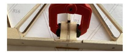
23) Stick 8MM balsa wood on the front end of the aileron and polished into triangles.
