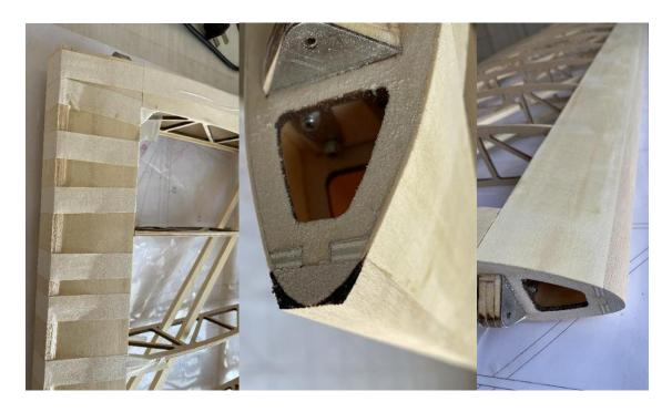
20) Stick balsa wood at aileron connecting rod exit.
