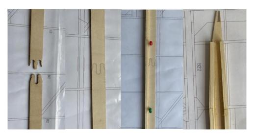
2) Stick the reinforcing board in front and middle of girder.
