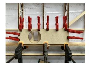
14) Stick balsa wood onto the front wing girder and smooth it.
