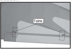
4) Deflect the aileron and completely saturate each hinge with thin C/A glue. The ailerons front surface should lightly contact the wing during this procedure. Ideally, when the hinges are glued in place, a 1/64" gap or less will be maintained throughout the lengh of the aileron to the wing panel hinge line.
