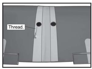
4) Attach servo lead to the aileron servo. Attach the string to the servo lead and carefully thread it though the wing. Once you have thread the lead throught the wing, remove the thread so it can use for the other servo lead.
