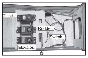
5) Install adjustable servo connector in the servo arm.
