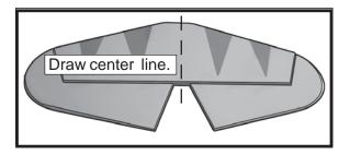
2) Slide the stabilizer into place in the precut slot in the rear of the fuselage. The stabilizer should be pushed firmly against the front of the slot.
