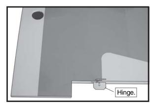
3) Slide the aileron on the wing panel until there is only a slight gap. The hinge is now centered on the wing panel and aileron. Remove the T-pins and snug the aileron against the wing panel. A gap of 1/64" or less should be maintained between the wing panel and aileron.
