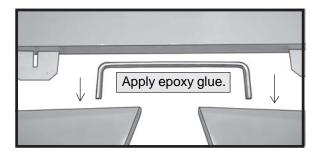
Glue the elevator hinges in place using the same tectniques used to hinge the ailerons.
