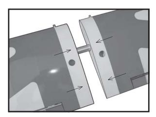
Apply masking tape at the wing join to hold the wing halves together securely.
