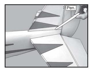
4) Remove the stabilizer. Using the lines you just drew as a guide, carefully remove the covering from between them using a modeling knife.
