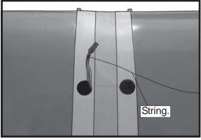
5) Tape the servo lead to the wing to prevent it from falling back into the wing.
