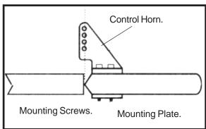
3) Position the rudder control horn on the left side of the airplane. Mount the control horn parallel with the horizontal stabilizer.
