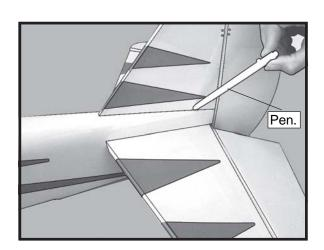
4) Remove the stabilizer. Using a modeling knife, remove the covering from below the lines you drew. Also remove the covering from the bottom edge of the stabilizer and the bottom and top edges of the filler block. Leave the covering in place on the sides of the filler block.
