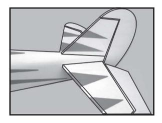
3) While holding the vertical stabilizer firmly in place, use a pen and draw a line on each side of the vertical stabilizer where it meets the top of the fuselage.
