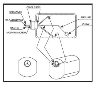
Attach the silicone fuel and pressure pipes to the tank. The lower pipe is the 'feed' and the upper two the 'pressure and fill'. The fill pipe is the next pipe.
