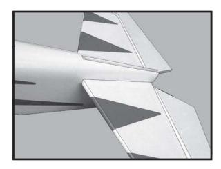
3) With the stabilizer held firmly in place, use a pen and draw lines onto the stabilizer where it and the fuselage sides meet. Do this on both the right and left sides and top and bottom of the stabilizer.
