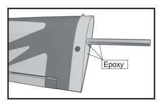
Carefully slide the two wing halves together and firmly press them together, allowing the excess epoxy to run out. There should not be any gap in the wing halves. Use rubbing alcohol and a paper tower to clean up any excess epoxy.
