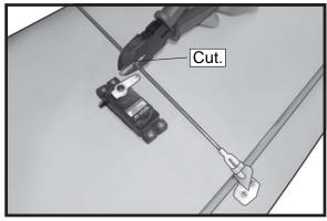
8) Make a 90-degree bend at the mark and cut off the excess wire leaving 10mm past the bend.
