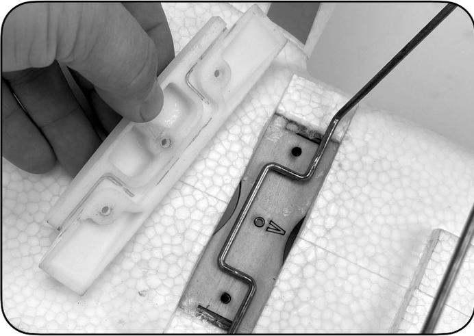
5. Place the front strut over the main landing gear mount in the fuselage. Use a #1 Phillips screwdriver and (3) M3x20 screws to secure the plastic bracket over the front float strut.
