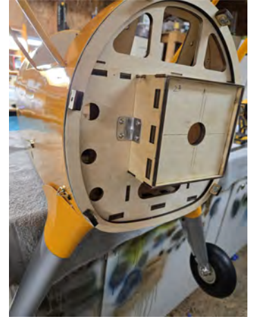
Engine Box reinforcements 4mm x 20mm phillips bolts
