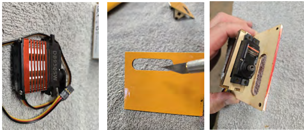
Wing servos high torque 400 oz min. 24 inch extension.
