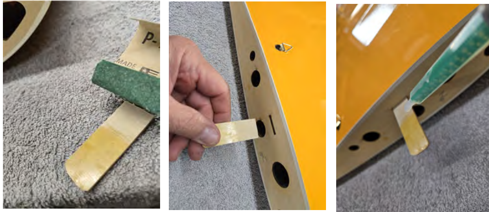
Top wing fiber glass attachment tabs using 2 part epoxy
