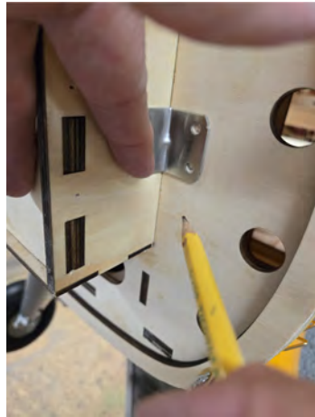
Engine Box reinforcements 4mm x 20mm phillips bolts
