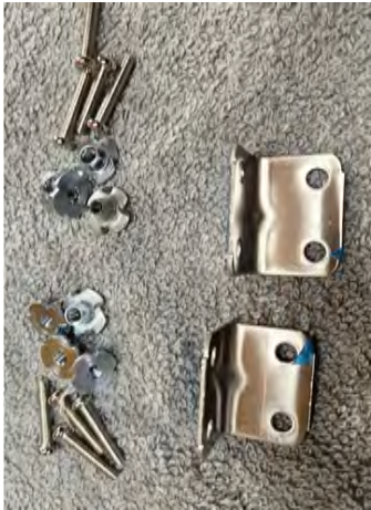
Engine Box reinforcements 4mm x 20mm phillips bolts
