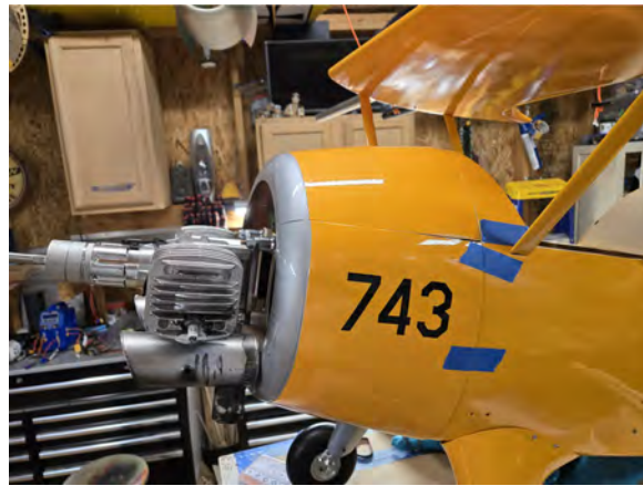
Cowling Bolts 3mm x 12mm bolts, washers, & O-rings
