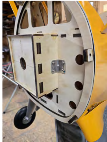
Engine Box reinforcements 4mm x 20mm phillips bolts
