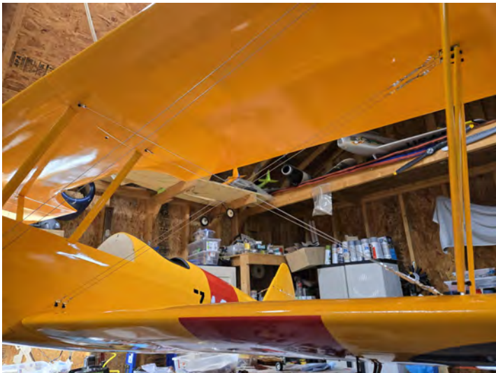
Flying wire connections 3mm x 20mm bolts and brass clips
