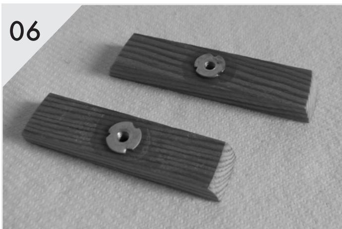
Attach in the back of the ridge a drive in nut and glue it with CA Glue.
