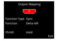
Press the SET button to select the output. On the next screen you can now define the output:
