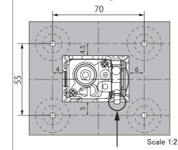
Be careful of contact between the fuel nipple and the firewall. Cracks in the fuel pipe can cause engine
