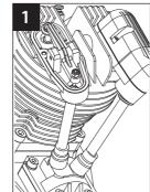
1. Remove the spark plug and rocker arm covers of a cylinder. Then turn the prop CCW by hand to place the piston at TDC of compression stroke.
