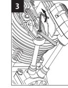
3. Once the gap is set, tighten the lock nut and attach the plug and covers.
