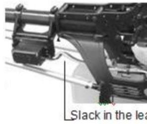
Fasten about 5-10cm from the servo outlet so that the lead wire is neat.
