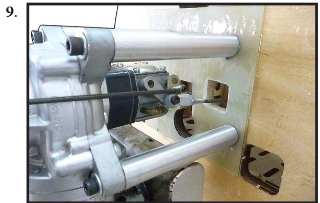
Position the engine with the drive washer (197mm) forward of the firewall.
