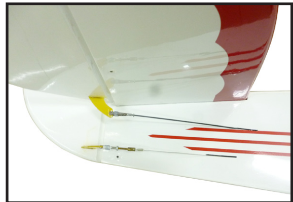
INSTALL BRACING WIRE AND METAL BRACKET AT THE TAIL.
