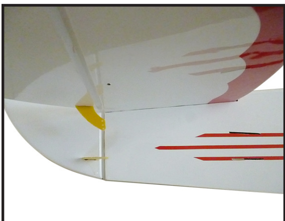
RUDDER PUSHROD HORN INSTALLATION.
