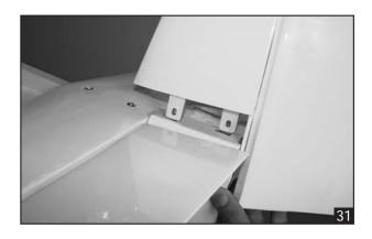
4. Remove the covering from the fuselage.
