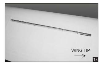
2. Install the air brake into the bay.
