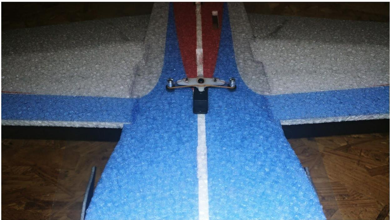
**After you electronically center your aileron servo by plugging it into your receiver and powering it on with zero sub trim and trim, you can glue it into the servo slot that is the most forward on the airframe with the output shaft facing rear. The aileron servo arm will be angled forward.**
