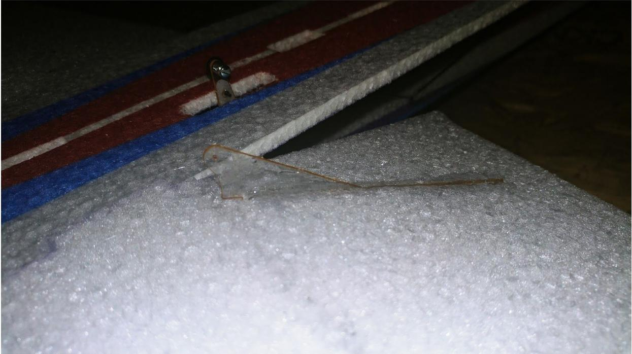
**Shown above is one of the aileron horns in place on the top of the aileron.**
