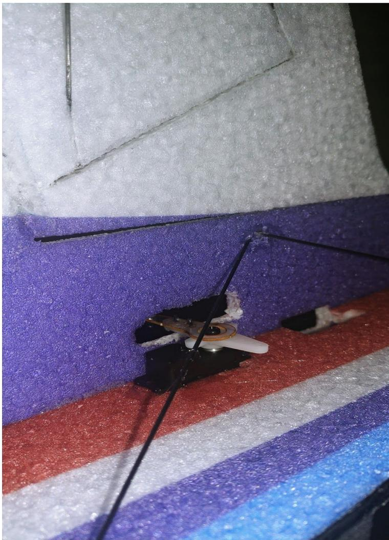
**Shown above is the glued in elevator servo. For the elevator, use the horizontal servo slot that is on the side of the fuselage. The arms used for the elevator and rudder servos are the singles. For both the elevator and rudder servos, face the output shaft towards the rear. For the MXS, position the servo arm towards the bottom of the airplane and run the linkage along the bottom part of the fuselage.**
