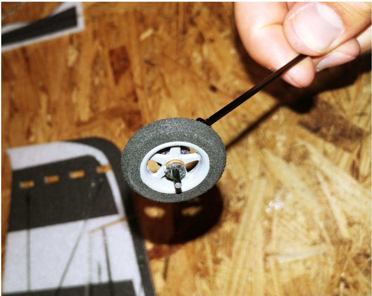
**Now locate the plywood/carbon fiber laminated collar to slide up next to the plastic wheel. Once again, do not apply glue yet as the tire will need to spin as freely as possible around the axle.**
