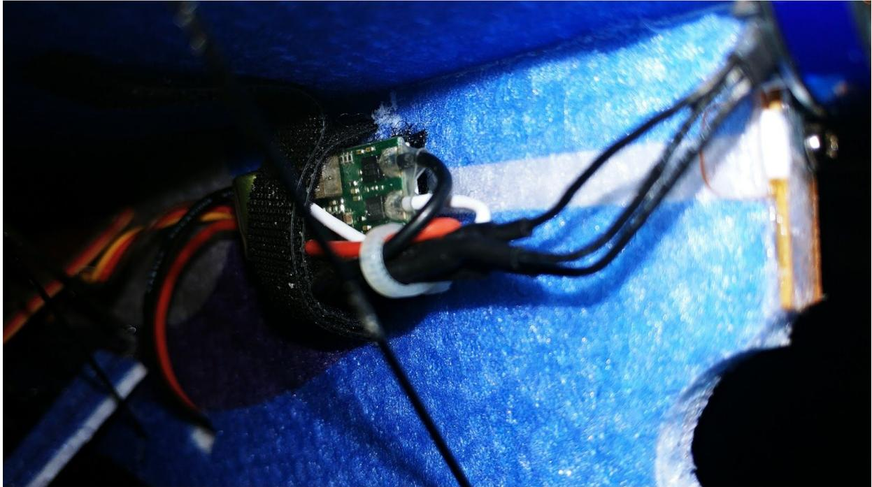
**Shown above is the ESC mounted using the velcro strap and a supplied zip tie is used to tie the ESC wires together.**
