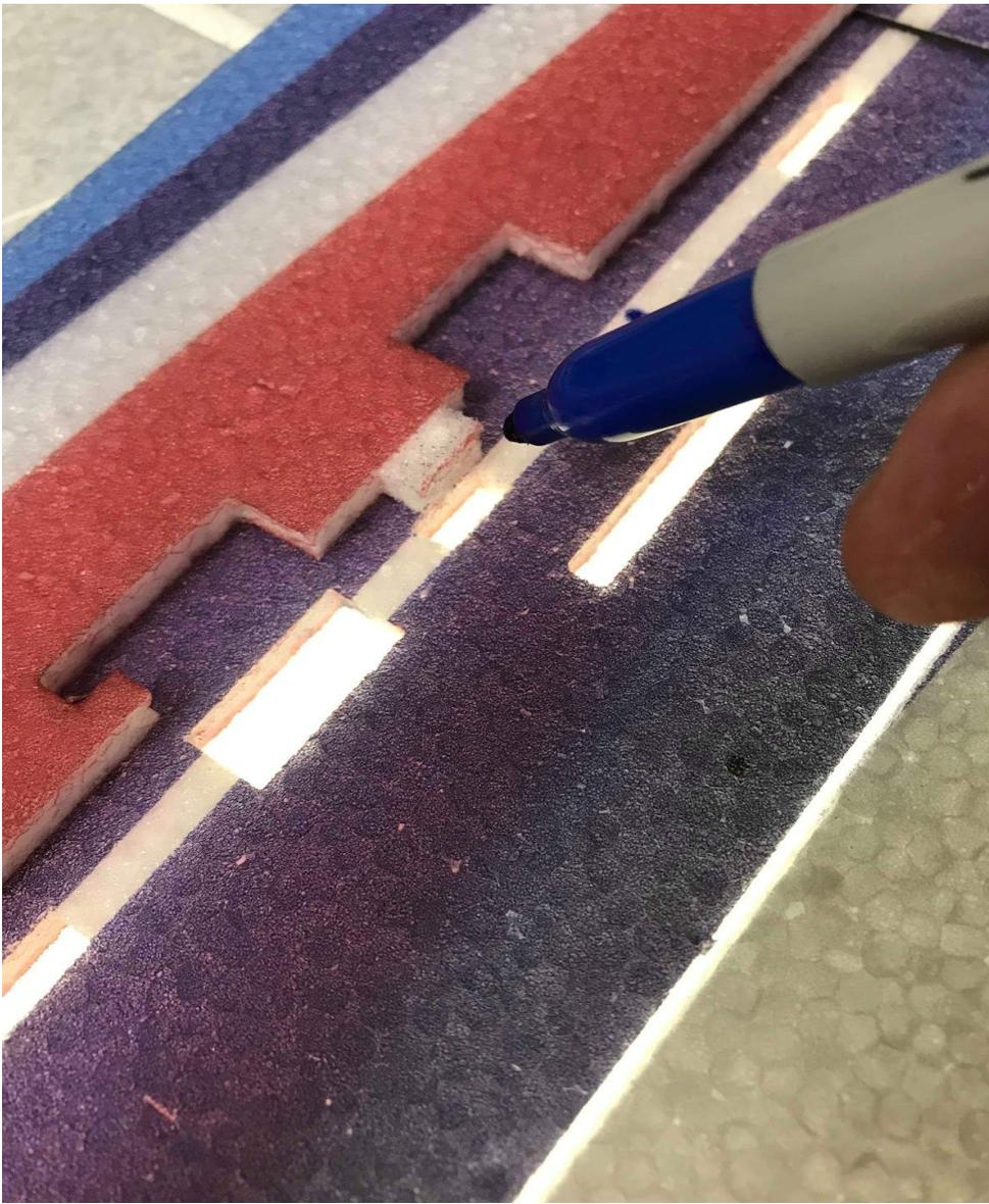
**If deciding to place glue on the horizontal part of the fuselage, you can mark out where the glue will be placed as shown above after test fitting the fuselage.**
