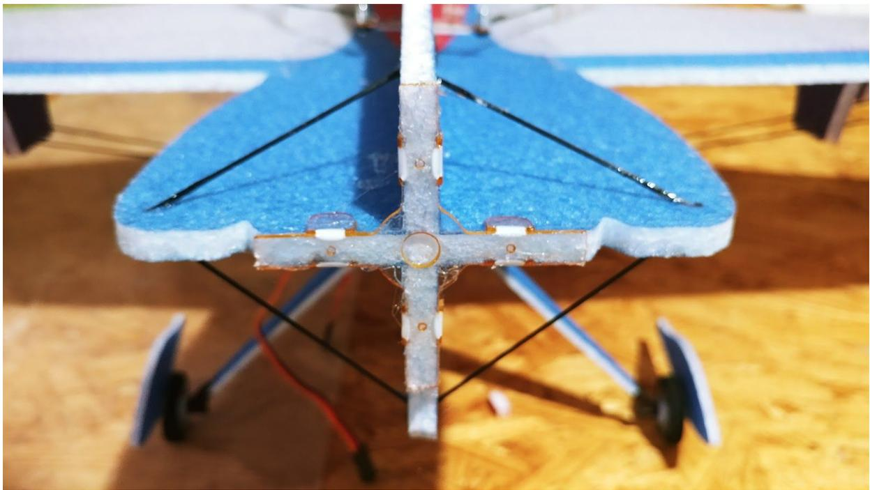
**Locate the motor mount as shown above. Test fit the motor mount to the front of the fuselage by bending the attached tabs 90 degrees and sliding it on without glue. Once test fitted, place adhesive on the inside of the motor mount covering every spot, then place again on the front of the fuselage making sure everything is flush and lined up correctly.**
