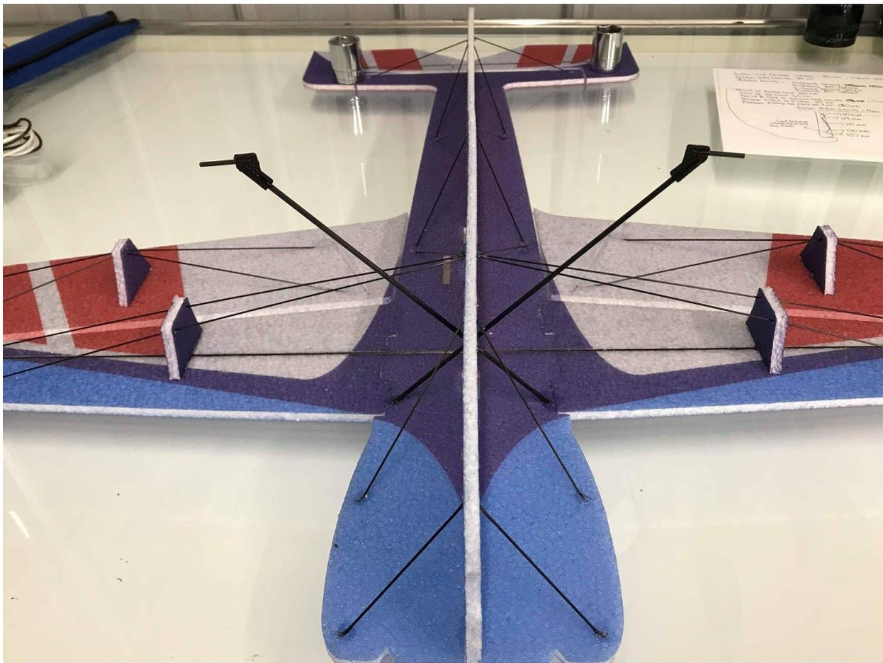
**Shown above is both landing gear legs in place. You will find the slots cut in the side of the bottom of the fuselage to slide each landing gear leg into. Make sure that the bottom of each leg is placed to where the airplane will sit level on the ground. Also shown is the first two carbon braces on the front of each side of the bottom of the fuselage.**
