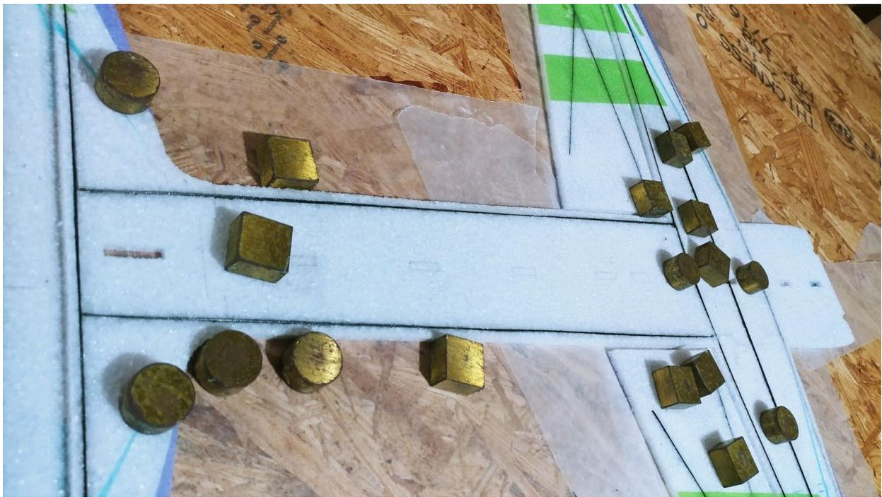
**The horizontal piece of the fuselage also uses flat carbon fiber spanning the entire length from the rear wing spar to the horizontal stab spar.**
