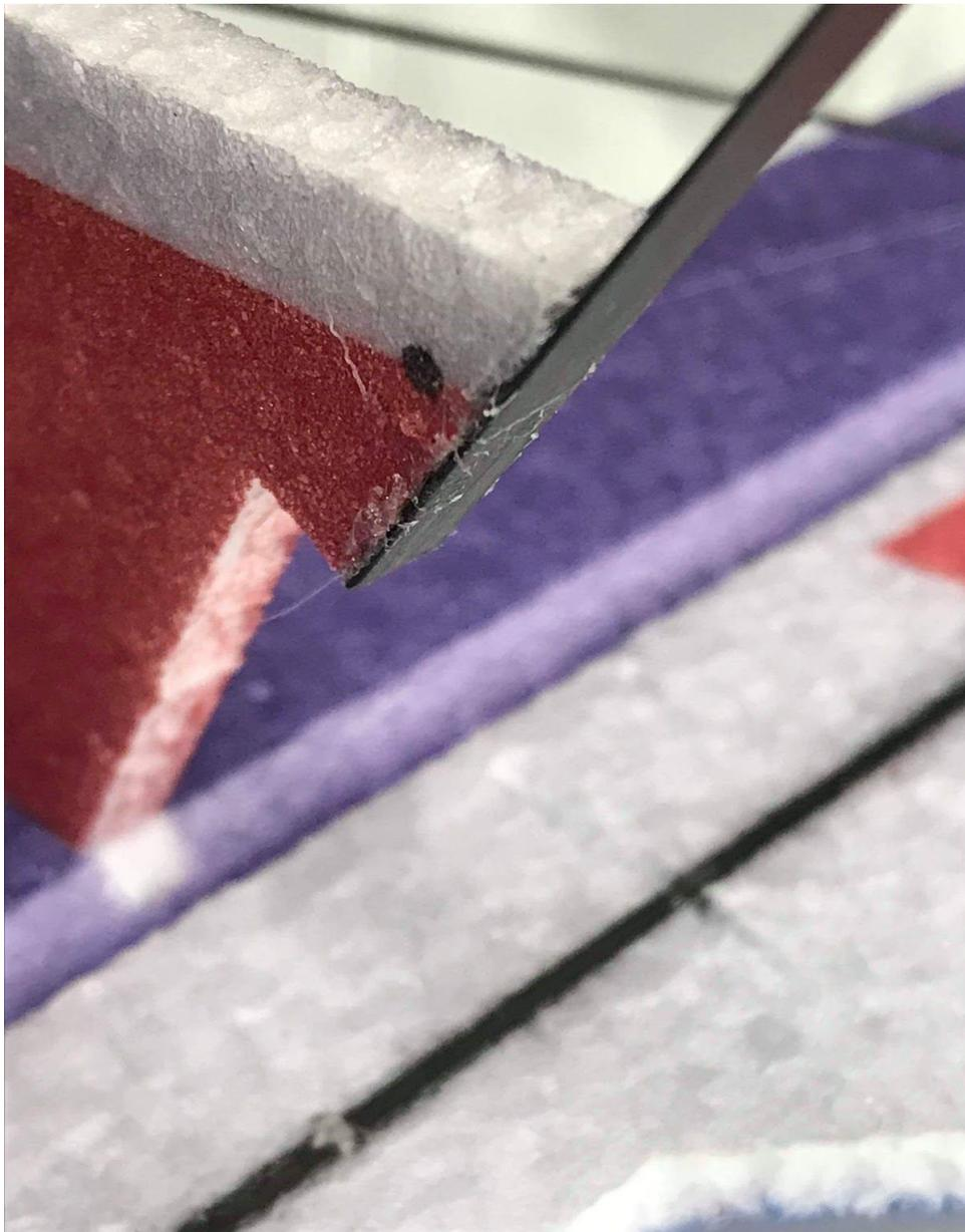
**Glue the tailpiece into place as shown above while making sure that it is on the same angle of the bottom of the fuselage to ensure that the airframe will sit level.**
