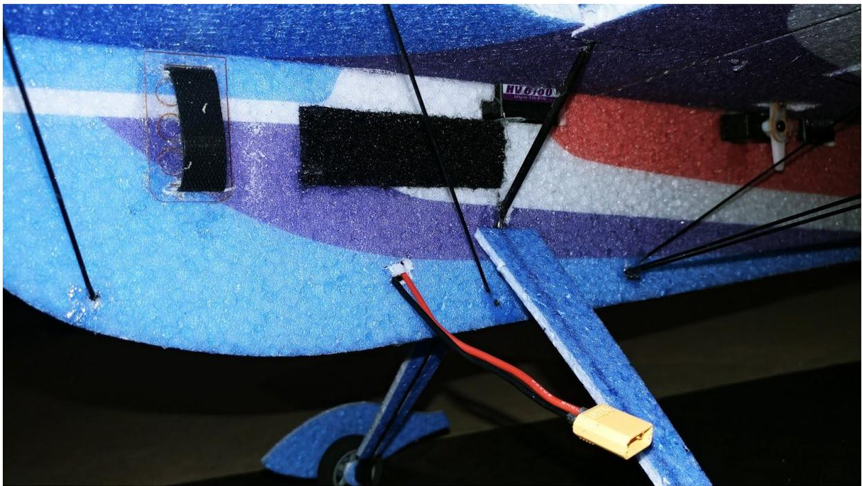
**The center of gravity and battery placement will depend on equipment used and personal flying preferences. The long piece of velcro mounted above is the location of the battery for this setup. To save space on the other side of the fuselage, the battery connector is put through to the opposite side of the ESC and receiver.**
