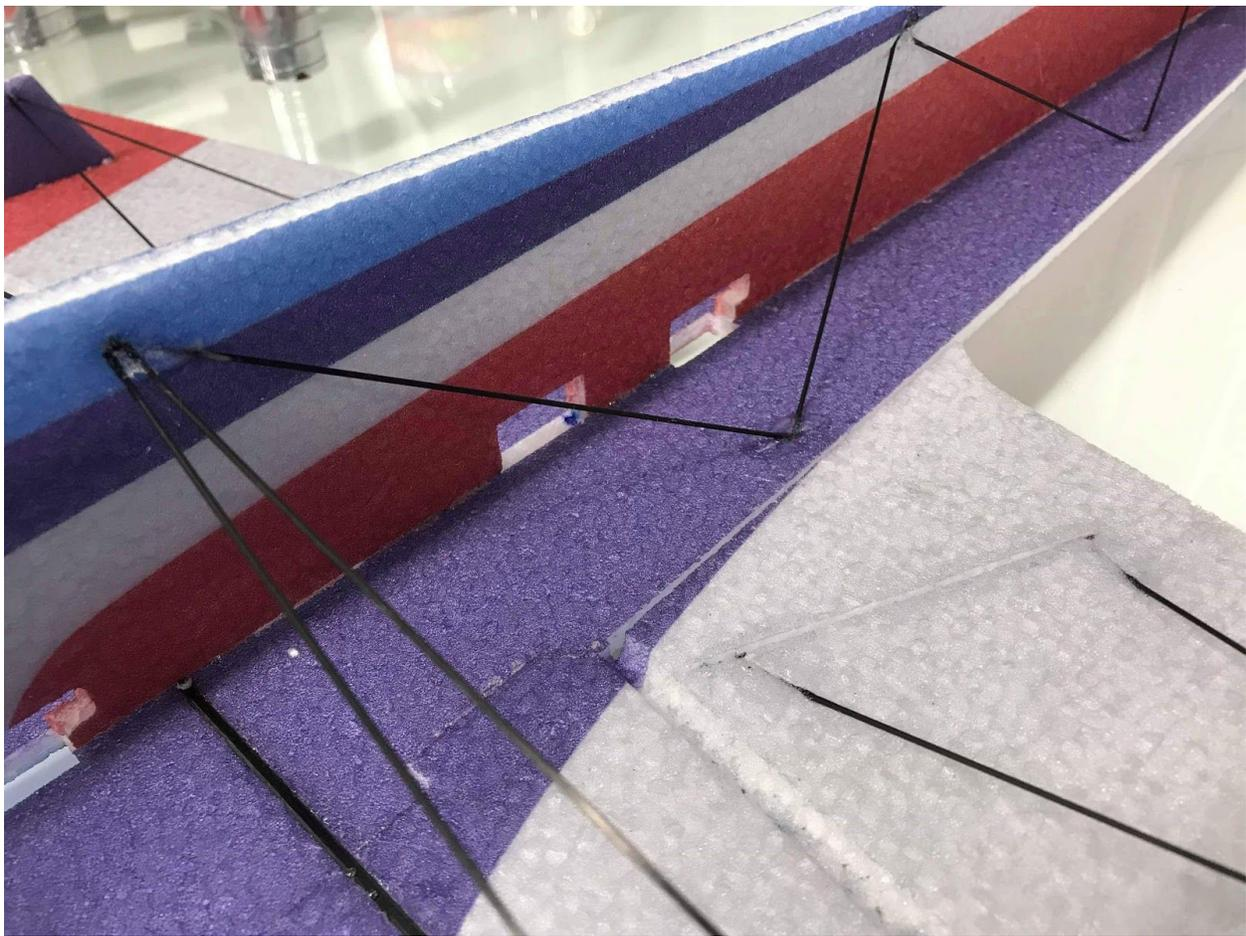
**Shown above is the rest of the bottom fuselage bracing up to the wing bracing.**
