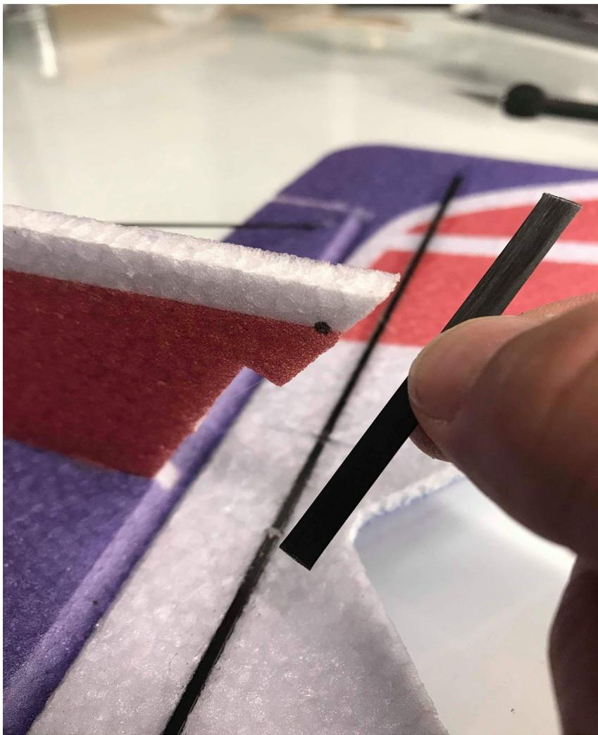
**Locate the short flat carbon fiber piece that will be used as the tail piece for taxiing, taking off, and landing.**
