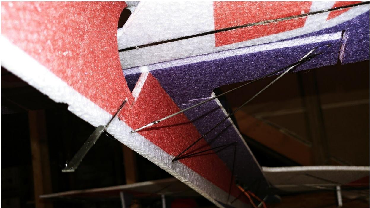
**Now that the top of the fuselage is glued in, you can glue the other rear carbon fiber rods to help strengthen the tail as shown above. They will be mounted**
