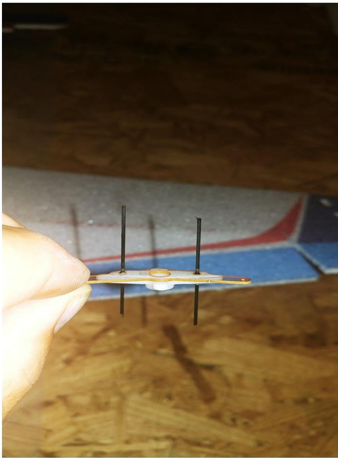
**You can now prepare your servo arms. Above is the provided double arm to be added on to the aileron servo arm that comes with the servo. Using the extension will provide the maximum amount of aileron throw. To join the two arms, use carbon fiber rods as shown above and glue them in through the holes lined up on each arm. It is important to use regular CA for this. You can then cut each rod down to shorten them. Another option is to use thread to join the two arms.**
