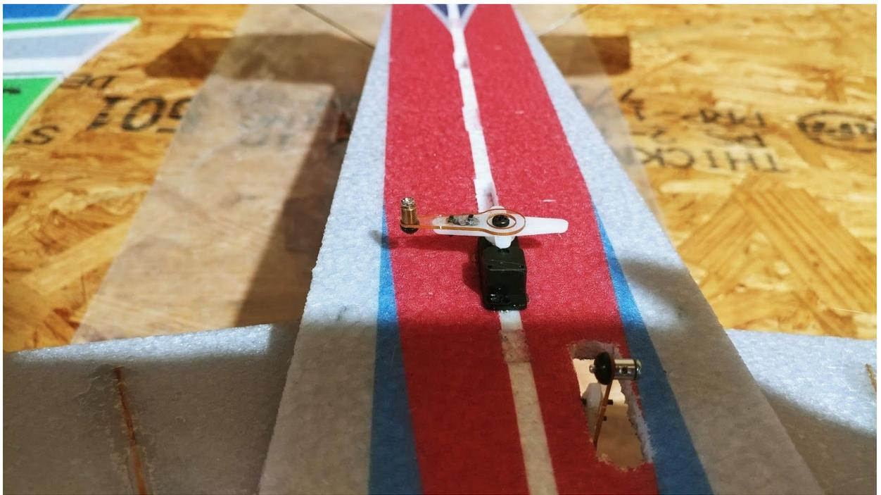
**Shown above is the rudder servo mounted.**
