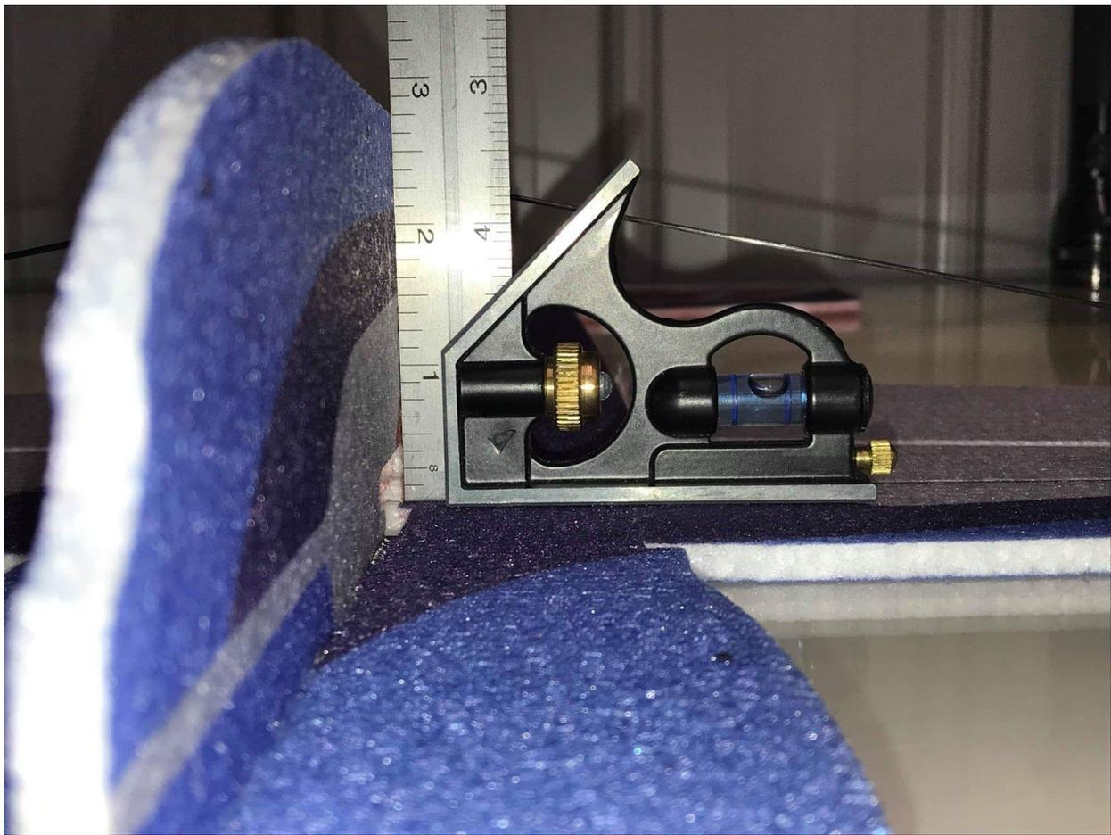
**It is extremely important to make sure that the bottom vertical part of the fuselage stays 90 degrees to the horizontal fuselage while the glue is setting. This can have a huge effect on the flying characteristics.**
