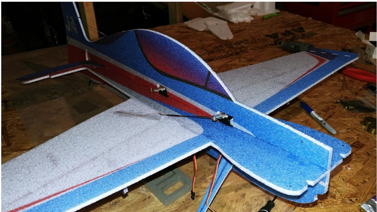
**Once the aileron and elevator linkages are set up, use the same process as gluing the bottom of the fuse to glue the top of the fuselage into place. Once again, it is important to keep this as straight as possible.**
