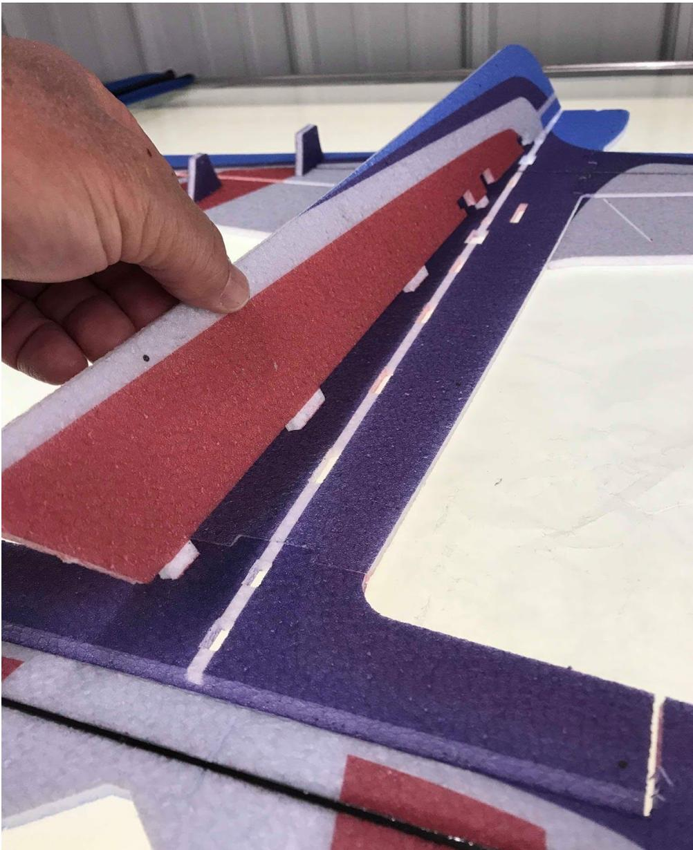
**You can now prepare the bottom half of the fuselage. Test fit this into each slot as shown above before glueing.**
