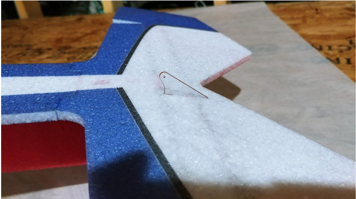
**The elevator control horn is the shortest and will be placed as shown above. You will notice a small square shaped cutout on the underside. This is meant to be placed around the spar of the elevator that was installed earlier.**
