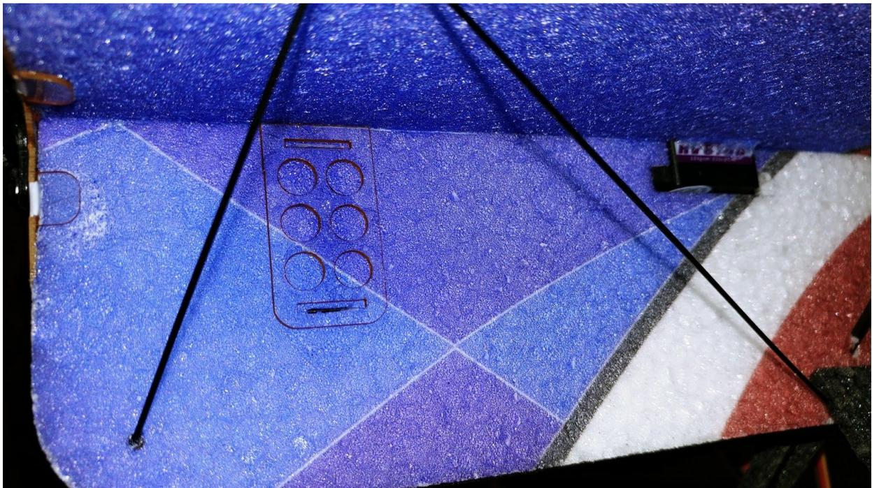
**The plate shown above is used to assist with the mounting the electronic speed controller. The plate will be glued on the opposite side of the fuse of where the ESC will be mounted. You will find the mounting location at where the slots are cut in the fuselage. If needed, slightly enlarge the slots after**
