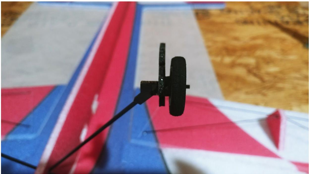
**Now, the tire/wheel is ready to be placed on the axle. Do not add any glue so that it can rotate freely around the axle.**
