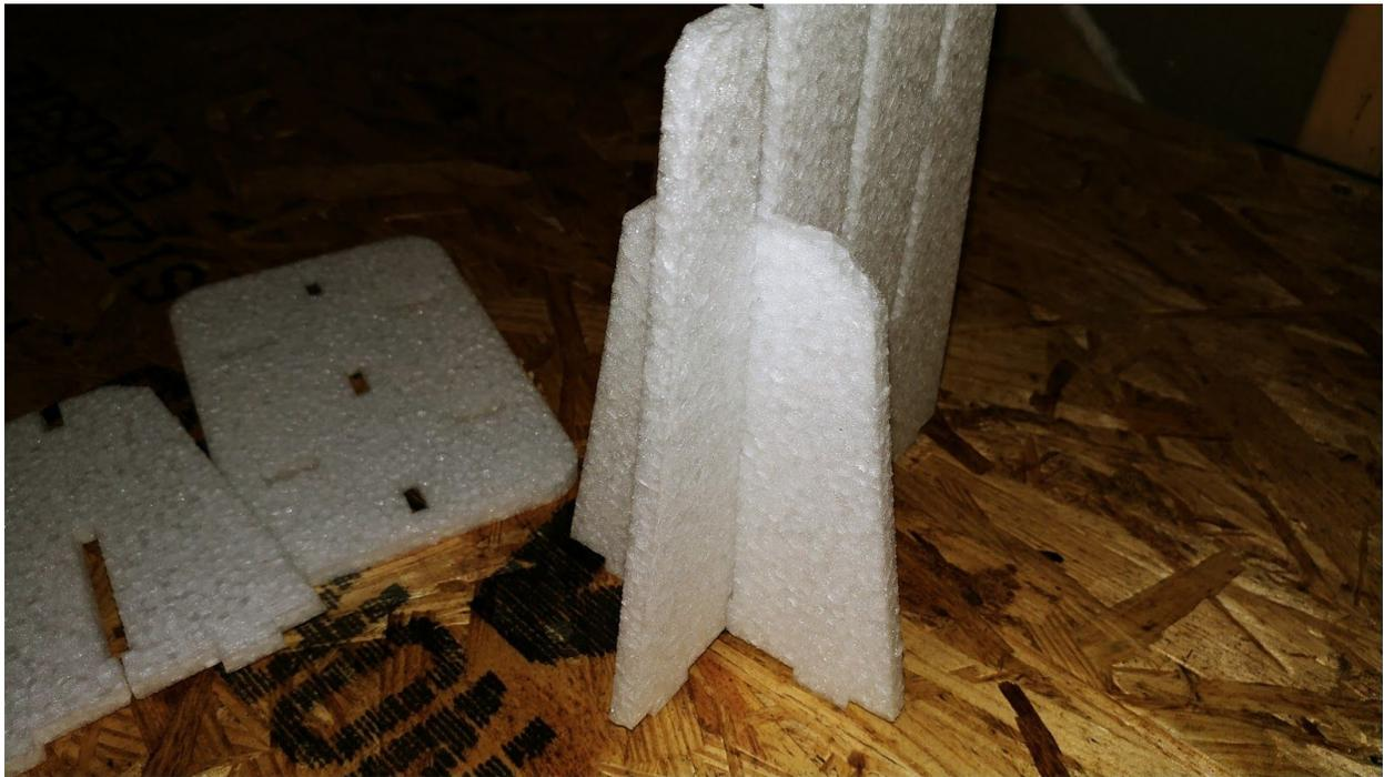
**Provided in the kit is the EPP stand used to slide over the fuselage. Assembly is shown as above.**
