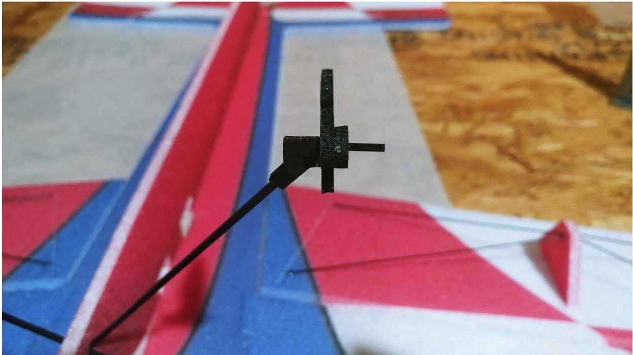
**Next will be sliding on the larger foam collar. Add just a small amount of glue to hold this into place against the wheel spat.**
