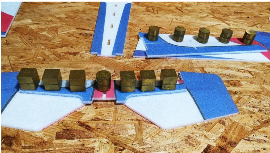
**In order to get consistent full range of all control surfaces during flight and setup, we recommend that the first thing you do after unboxing is weighing down the control surfaces as shown above. Each surface will take about**
