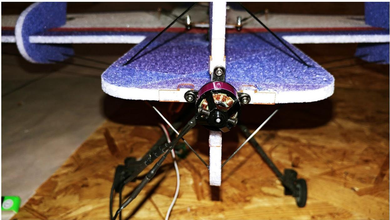
**Line up the holes in the motor mount that is mounted on the motor itself to the mount that is mounted on the airplane. If needed, pre drill the holes needed to mount the screws.**
