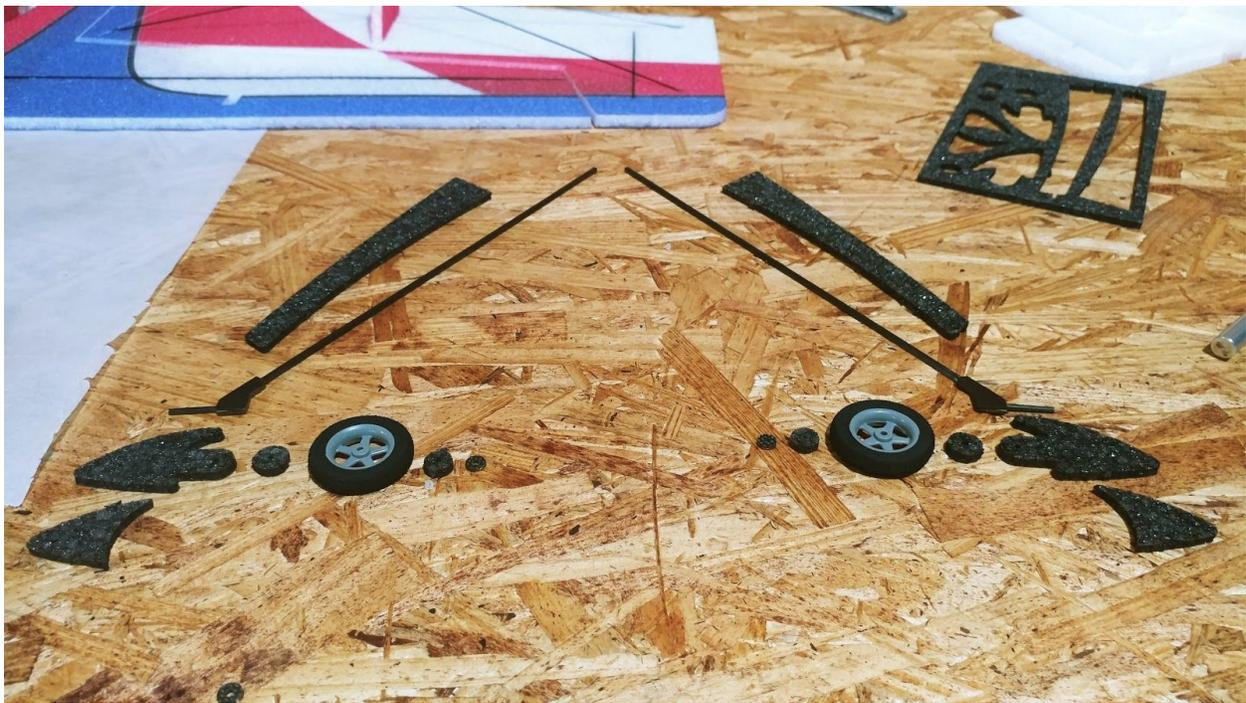
**Shown above is the entire assembly for the landing gear. The square carbon fiber landing gear is already glued into the axles. You will find the wheels as well as three total collars (2 foam pieces, and 1 wood/carbon laminated piece).**
