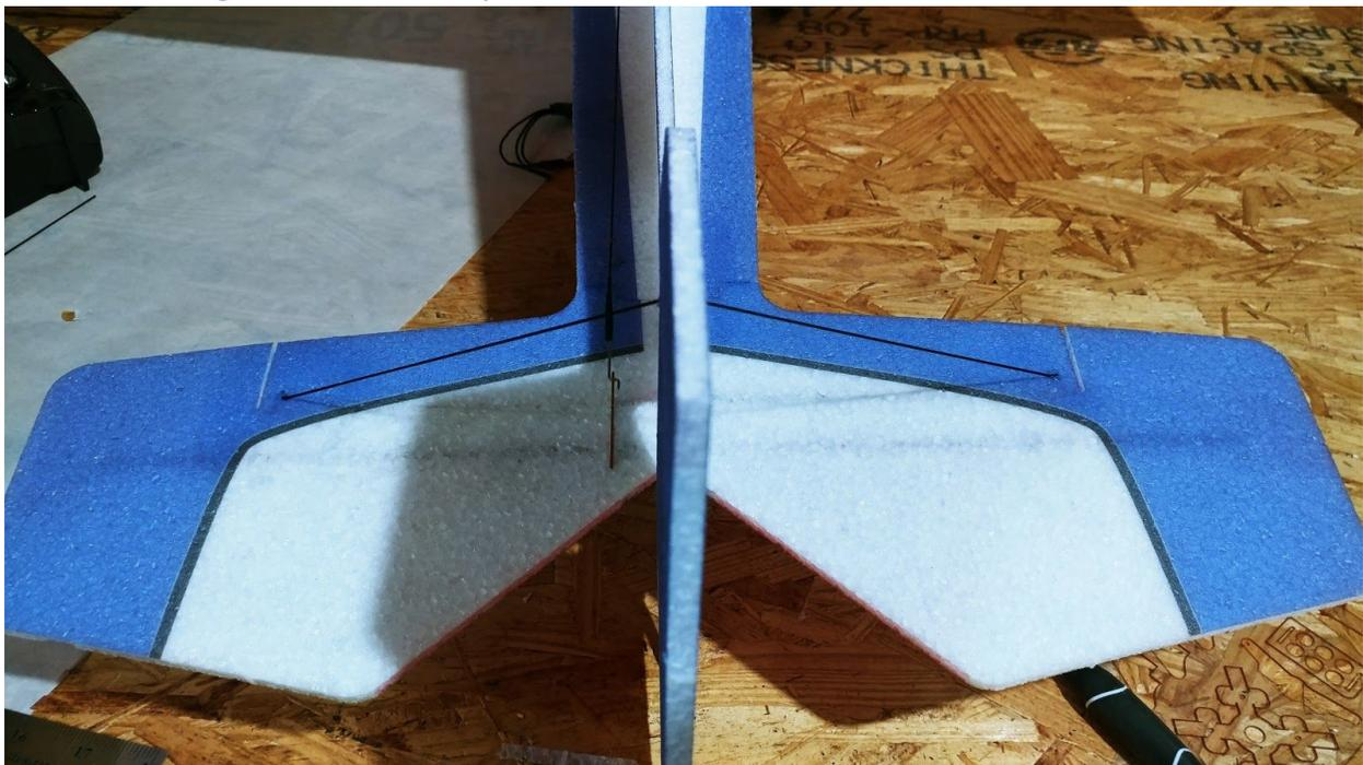
**For bracing of the top of the horizontal stab to the vertical stab, 2 180mm carbon rods will be used in the configuration shown above.**
