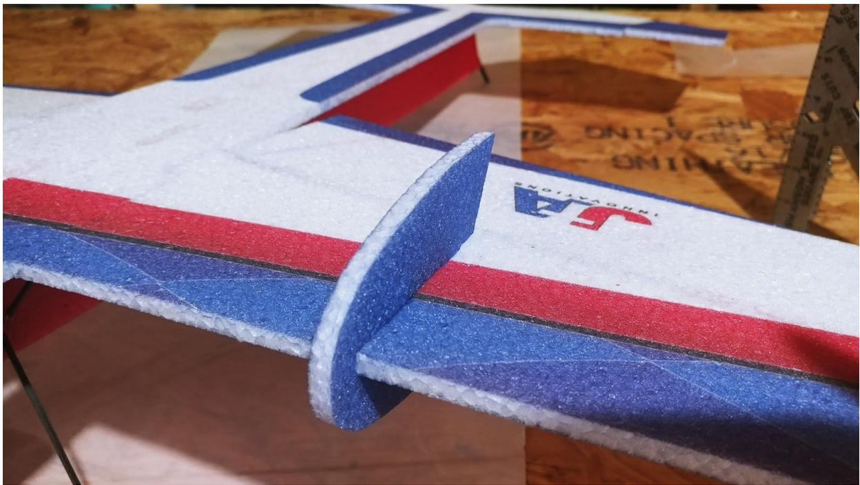
**Locate the 2 side force generators. You will notice that one side of each SFG has cut outs. Make sure that these cutouts are facing the bottom as this is where the carbon fiber bracing will be passing through on the bottom of the wing. Make sure that the SFG fits snug and flush with the wing. Apply glue to all 4 tabs, then repeat for the other wing.**
