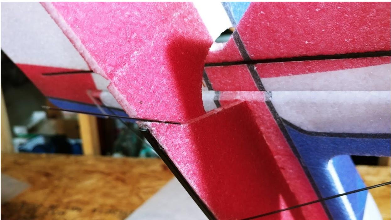
**Notice the joining of the top of the fuse to the bottom of the fuse at the point of the tailpiece. Make the connection so that the bottom of the fuse is one straight line all the way to the trailing edge of the rudder. This is because the amount of down elevator travel depends on the placing of this.**
