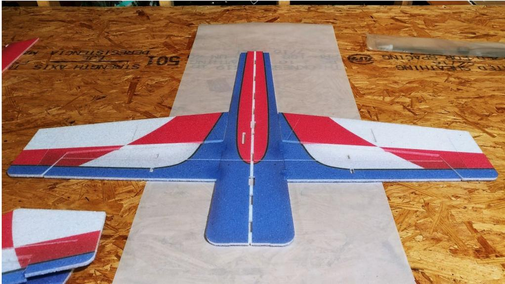
**Now, locate the horizontal piece of the fuselage as well as both wings. Make sure the fuselage is flat inverted and test fit each wing panel. After test fitting, you can now proceed to glueing in the wings to match up with the cutouts in the fuselage. We recommend using a sheet of wax paper or parchment paper to avoid the airplane becoming glued to the workbench.**
