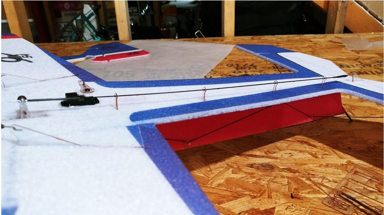
**Once the servo is centered, and both sides of the linkage are glued and tightened with heat shrink, you can now glue in place the guides for the linkage. It is best to put a small bit of glue inside the cutout then place in the guide. Make sure that they are all standing straight up and flush with the fuselage. If the linkage is getting stuck in one of the holes, use sandpaper on the linkage to ever so slightly slim the carbon.**
