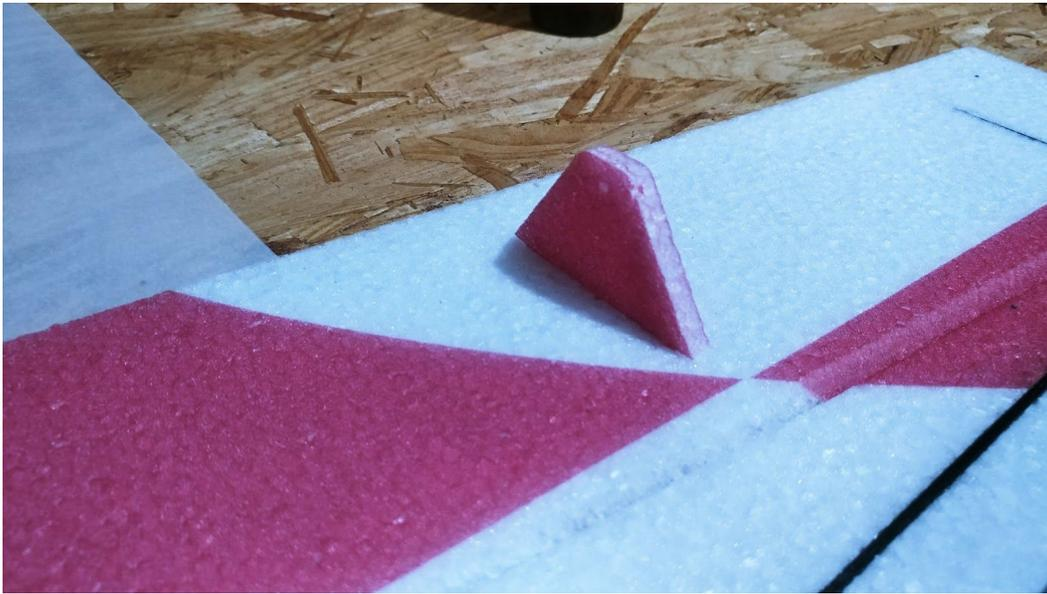
**Locate the triangular joiner that will be placed on the underside of each aileron. Once you make sure that it fits clean and snug into the cutout, you can glue this piece in and repeat to the other side.**
