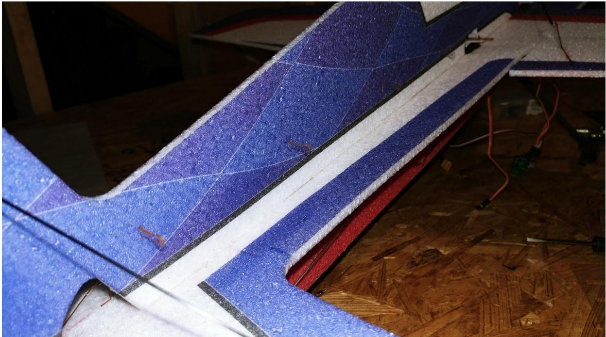
**The rudder servo linkage connection is now ready to be accomplished using the same technique as the elevator linkage. These guides will be mounted horizontally to the side of the fuselage. Just as the ones used for the elevator, you will see the cutouts pre made in the fuselage. Do not glue them in until the Z bend and straight link are both secured to the carbon linkage using REGULAR CA and heat shrink.**
