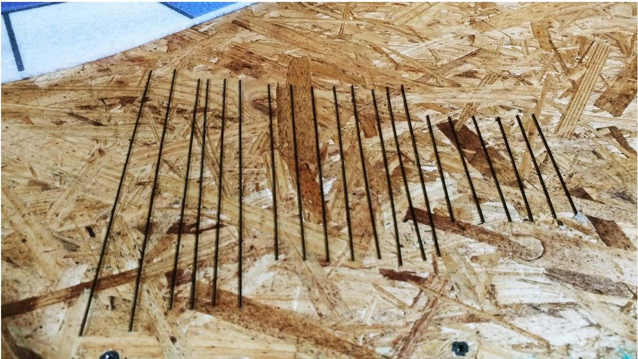
**Shown above is the carbon fiber arrangement that will be used to brace the fuselage. Most will be used for the underside, but some will be used for the top in a later step.**
