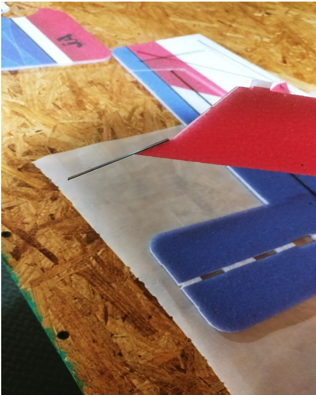
**As shown in the photo above, a flat piece of carbon fiber will be used for the tailwheel purpose and allow the aircraft to rest and taxi on the ground without coming in contact with the foam. This will be glued to the bottom vertical piece of the fuselage. The length of this piece is 60mm.**
