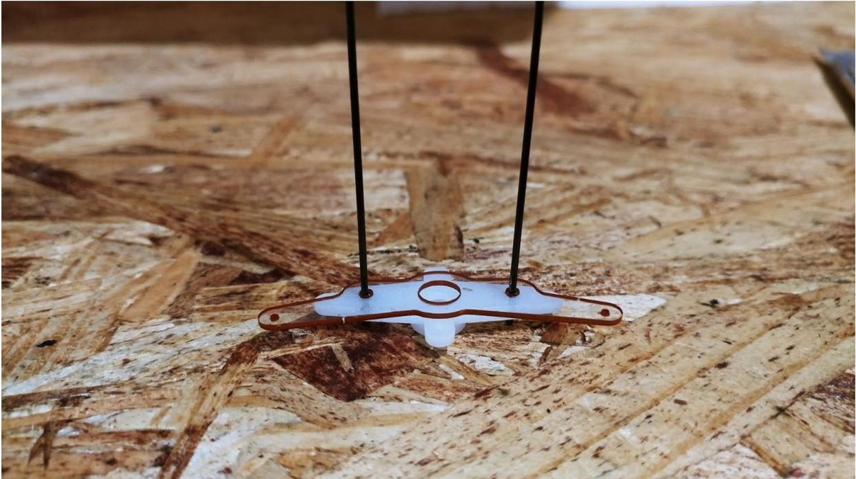
**In order to extend the length of the servo arm to provide maximum travel to the control surfaces, you may be interested in using the supplied servo arms. Glueing them to the plastic arms that are provided with the servos will**
