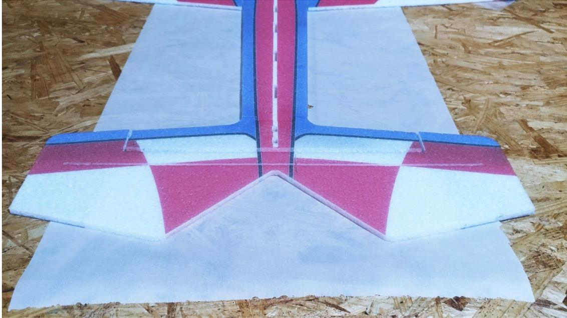
**Test fit the horizontal stab/elevator into the rear of the fuselage. If all is well, glue into place making sure that it is flush with the fuselage and flat with the rest of the airplane.**
