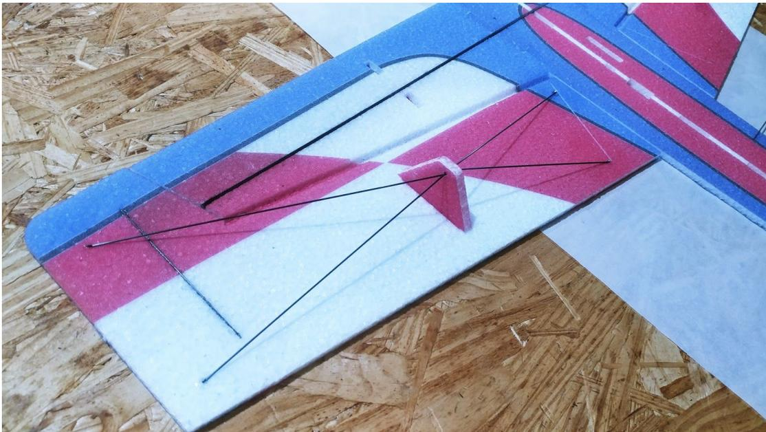
**With the joiner in place, you can now begin the process of bracing the aileron. This will include four carbon fiber rods in the configuration shown above. The lengths for each are 190mm, 170mm, 140mm, and 155mm. The carbon rods will**
