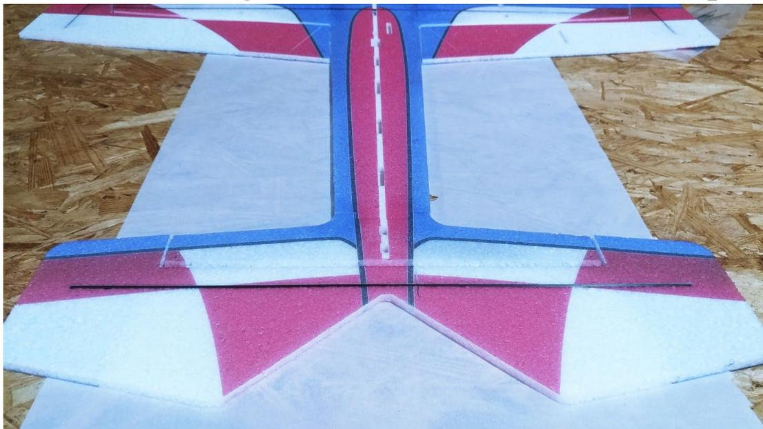
**Locate the carbon fiber elevator spar. It will be square just as the wing spar is and cut to fit the cutout in the elevator. Length will be 400mm.**
