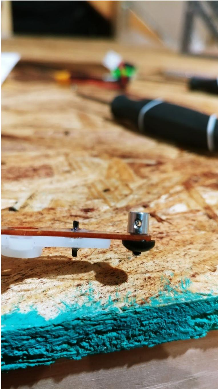
**The mini EZ connector as shown above will be used to connect the linkage to the servo arm. It will be easiest to place these on the arm while it is off of the servo. Put the top**
