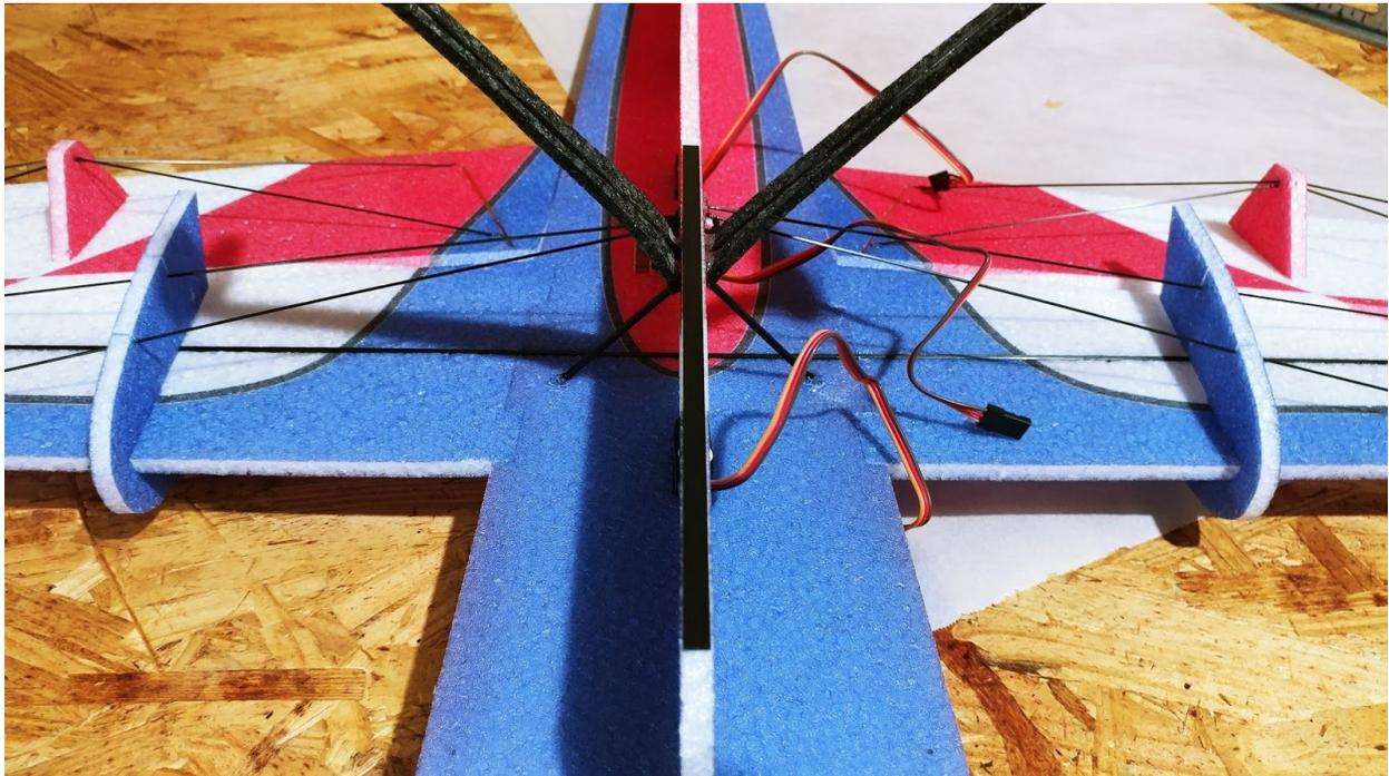
**This 190mm flat carbon fiber piece will be used to strengthen the bottom of the fuselage from the front of the fuse through the landing gear location.**
