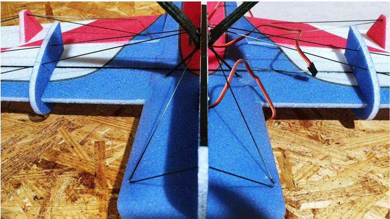
**Shown is the configuration for the underside bracing of the “cowling” area. The two most forward pieces are 80mm, and the pieces that extend to the landing gear are 145mm.**
