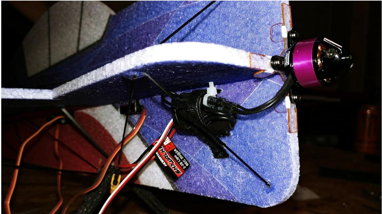
**Shown above is the ESC side, the opposite side is where the plate was mounted. Notice the velcro strap coming through the fuselage and around the ESC. A small piece of velcro may be needed to mount the ESC directly on the foam as well for the best possible strength.**
