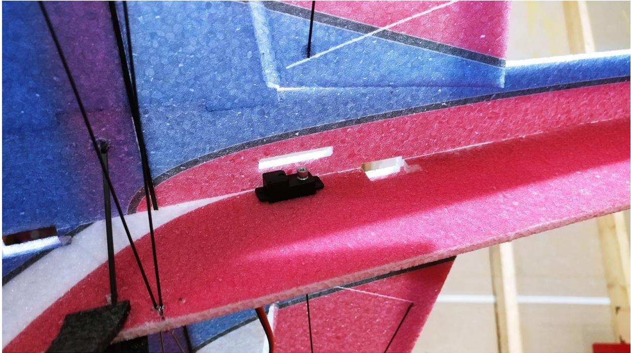
**This is the location for the elevator servo. It will be placed between the aileron and rudder servo and on the underside of the fuselage. The servo arm will be pointed up as the control horn will be placed on the top of the elevator.**
