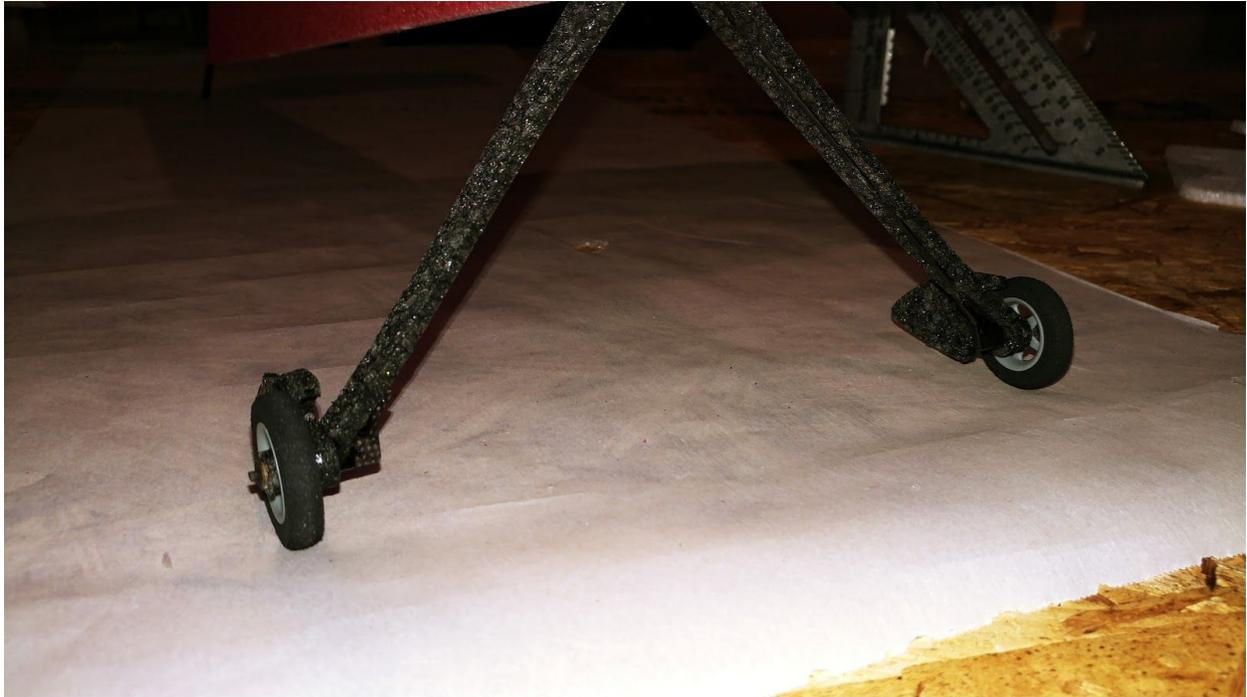
**Now, you can apply the foam landing gear covers. Once you make sure that the carbon fiber rod of the landing gear is fully inserted into the slots, you can apply glue to the connection at the bottom of the cover as well as at the top where it joins the fuselage. Also, make sure to put glue along the landing gear to ensure the covers will stay flush.**
