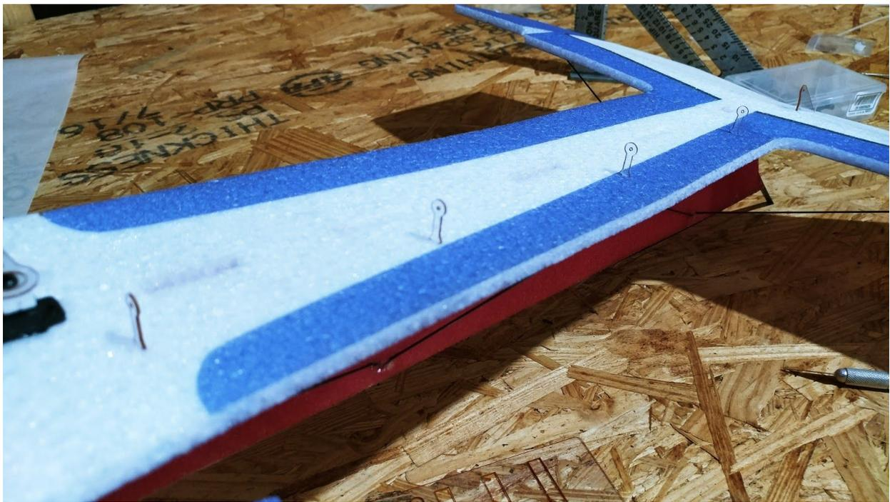
**For the elevator linkage, test fit the small guides into the cutouts as shown above. There are 8 total in the kit (4 for elevator, 4 for the rudder).**
