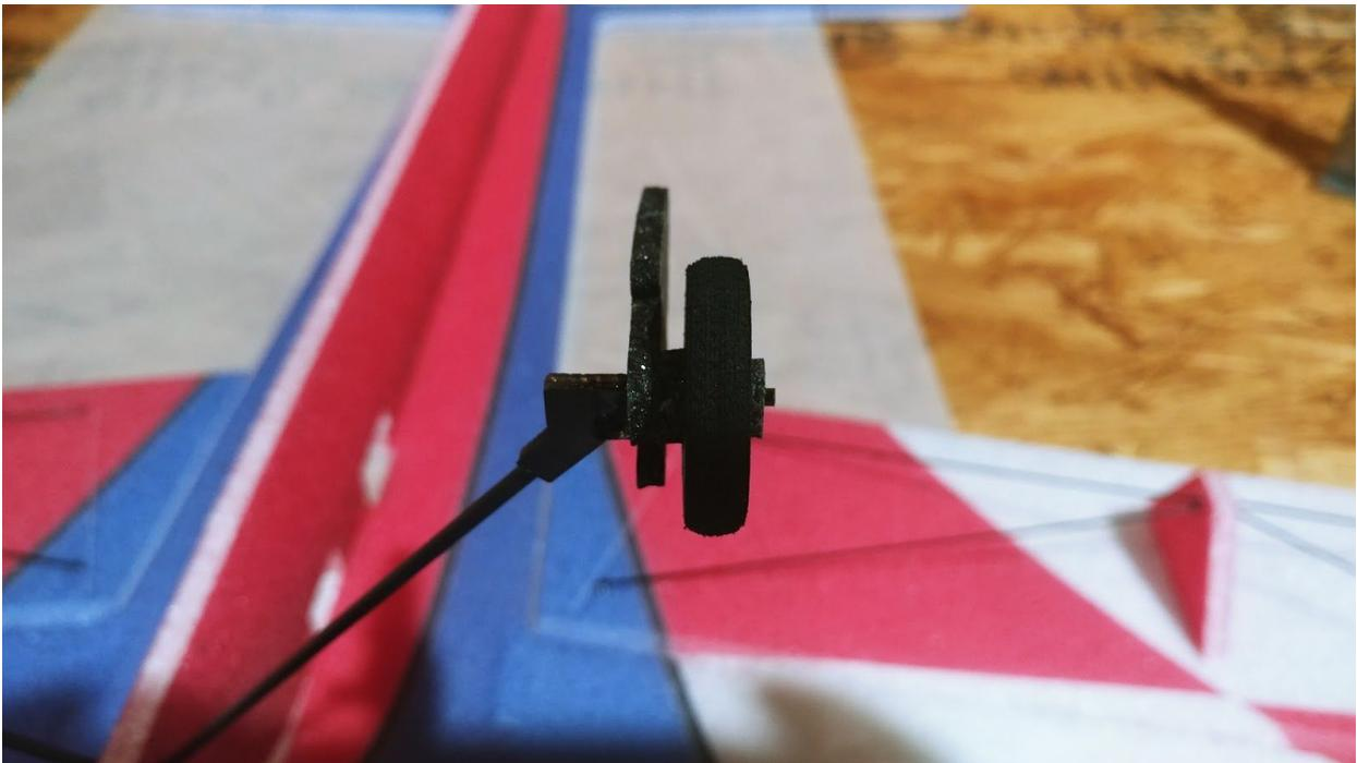
**Next, slide on the smaller piece of foam that will act as the collar on the outside of the wheel. Once again, do not add any glue to this piece.**
