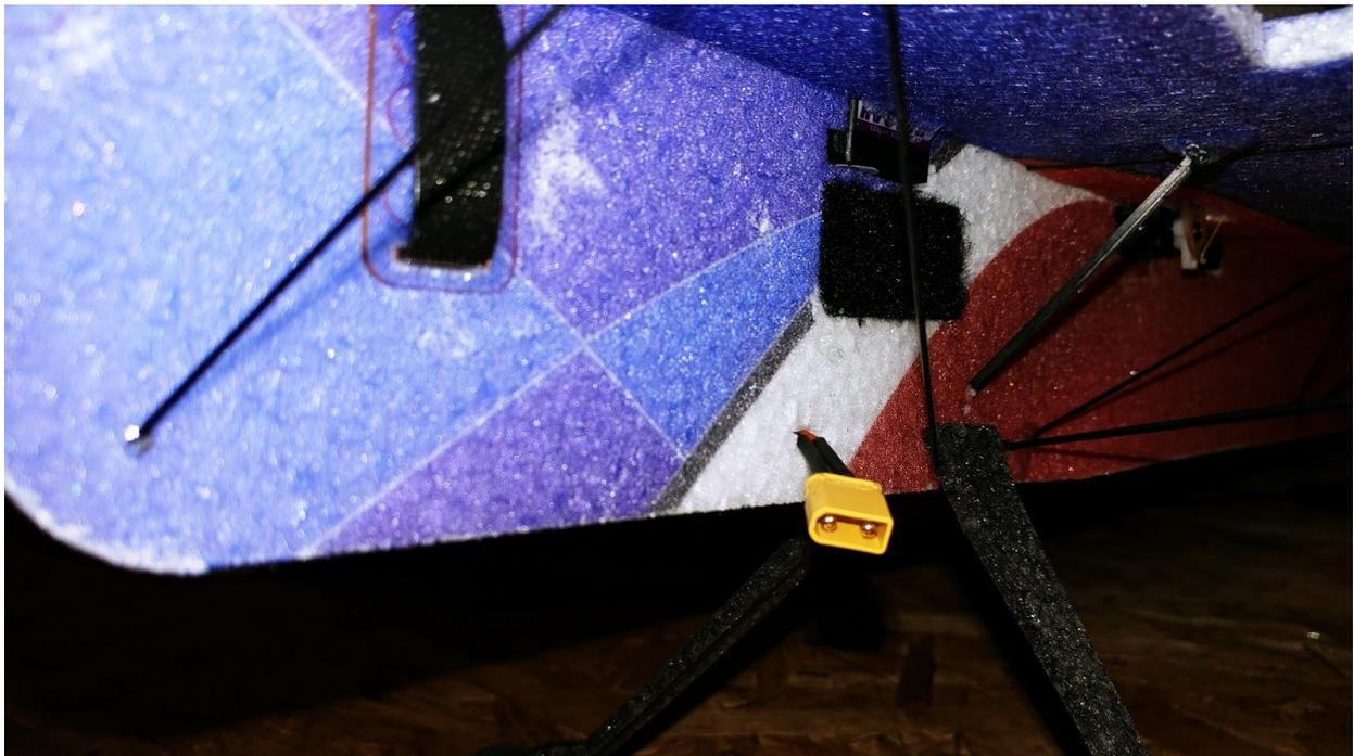
**If you would like, the battery can be mounted on the opposite side of the receiver and ESC to save some space. To do this, simply cut a small hole into the foam and and guide the connector through to the battery side of the airplane.**
