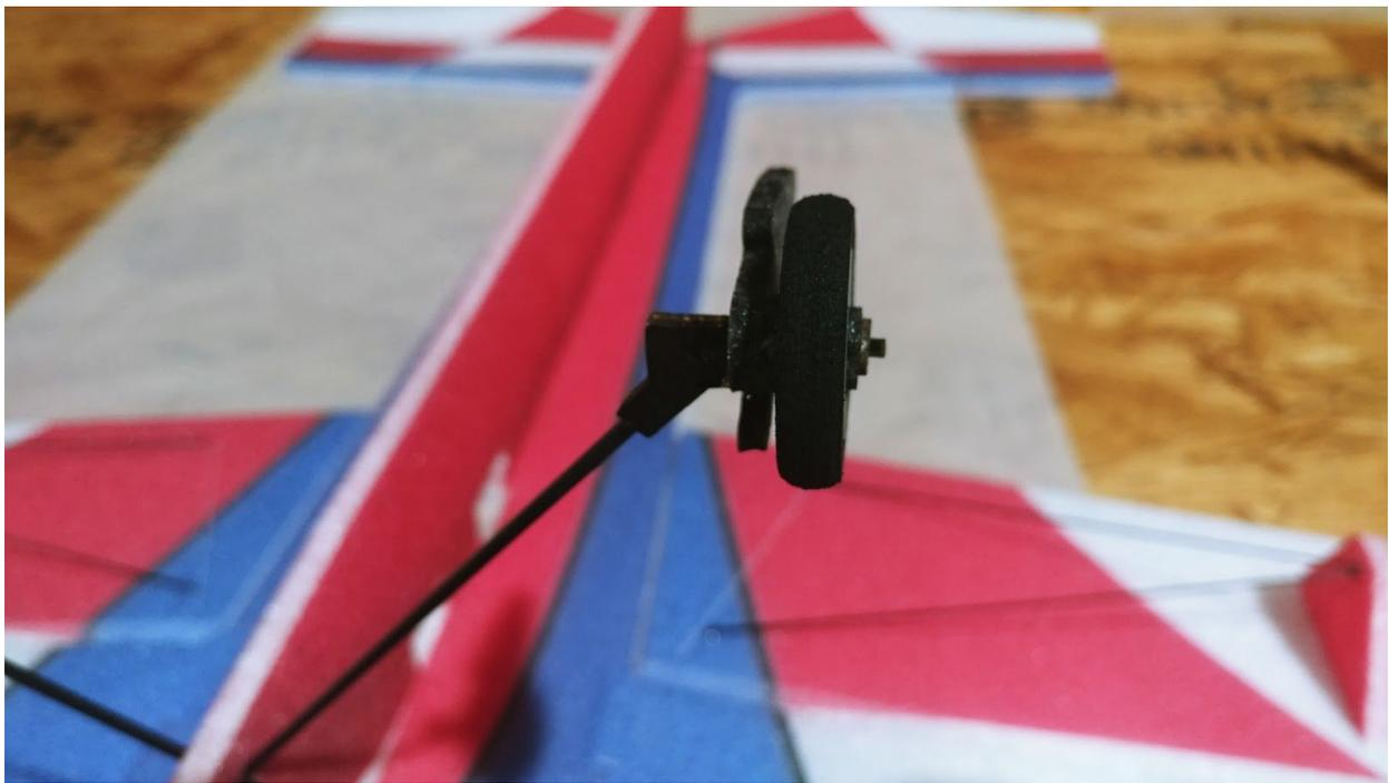
**Lastly, apply the small wooden collar that will hold the wheel onto the axle. You can add a small drop of glue to ensure that this piece will not slide off.**
