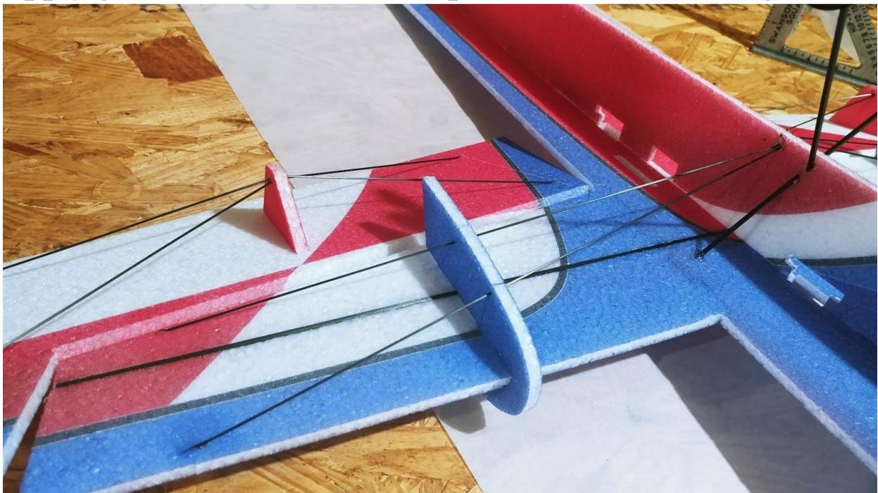
**This is the configuration for the wing bracing. In total, there are 2 pieces of carbon fiber used per wing to accomplish this.**
