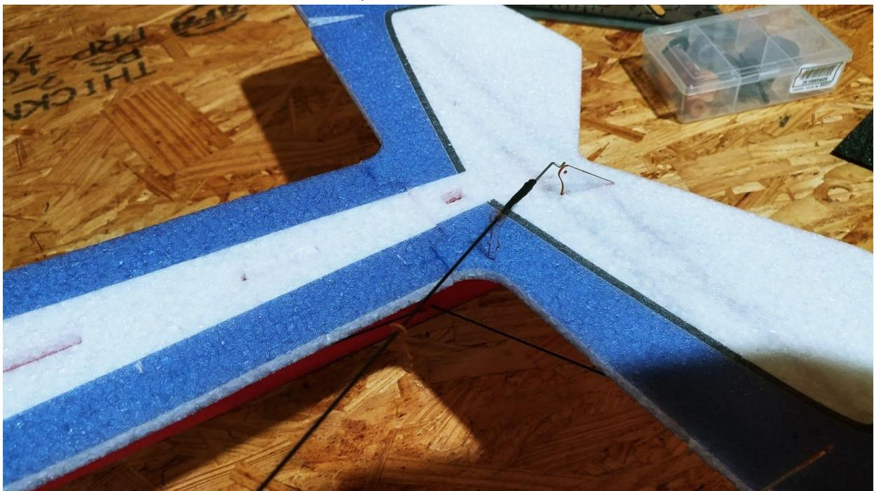
**Shown above is the elevator linkage connected to the Z bend using the same process that was used for the aileron (CA, then heat shrink over top). Also notice the guides for the linkage are slid over the linkage but not yet glued in. They will be glued in once the centering is done and the linkage is**
