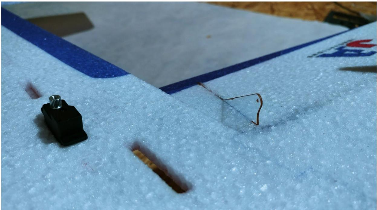
**The control horns will be placed and glued into the slots of the appropriate control surfaces. Make sure when applying the control horns that they are flush and that the hole for the linkage is directly above the hinge line. It may be a good idea to scuff the sides of them with sandpaper. Shown above is one of the aileron control horns.**
