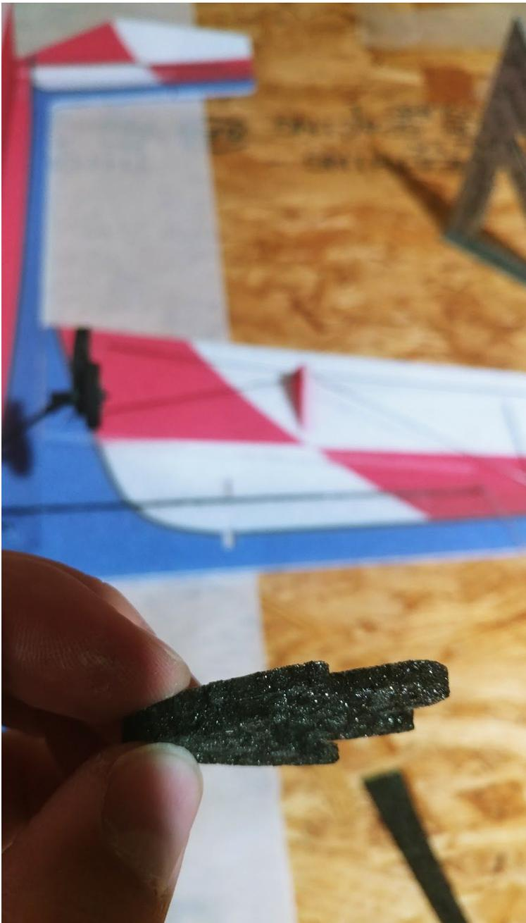
**Along with the EPP wheel spat, there is an additional piece of EPP that is the same shape that will be glued together to provide strength for the rear part of the spat. The photo above shows the two pieces glued together.**
