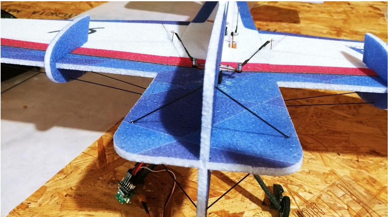
**Once the top fuselage is fully glued in place, the bracing for the top can be started. Shown above are the two 80mm carbon rods used for forward bracing of the aircraft.**
