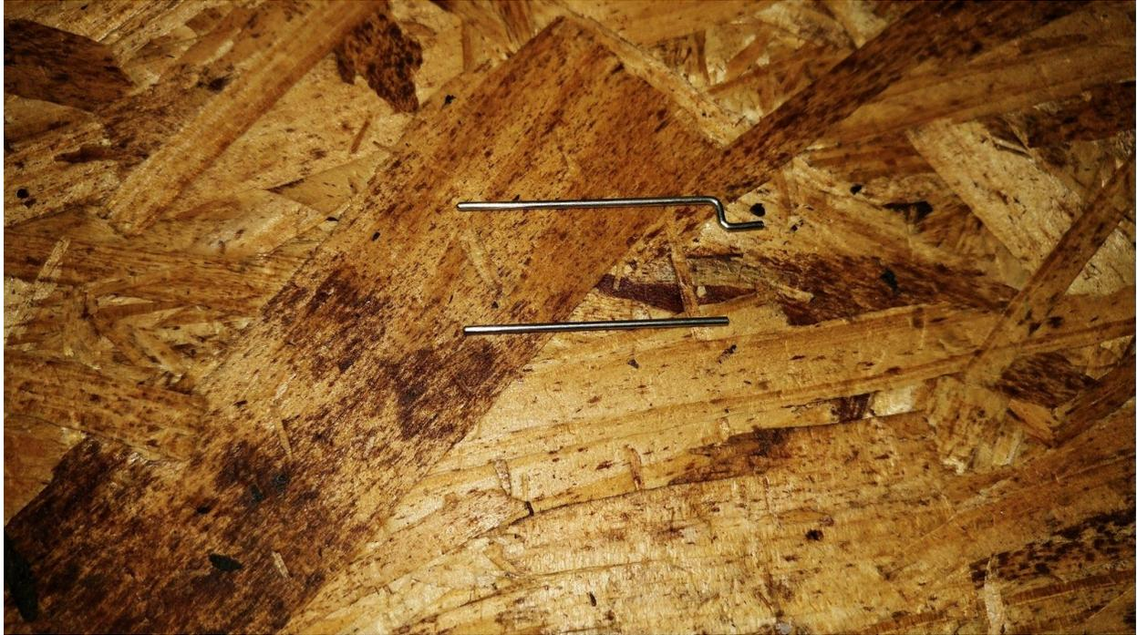
**Above are what will be used for each end of the control linkages. The Z bend will be inserted into the control horn while the straight end will be slid into the opening of the mini EZ connector on the servo arm.**
