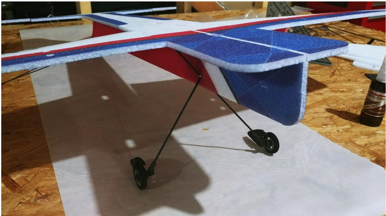
**Pictured above is the landing gear mounted on the airplane. You will notice that each landing gear side is crossed through to the opposite side of the airplane. You should be able to find two slices in the vertical fuse that will indicate where the carbon landing gear will slide through. Make sure**
