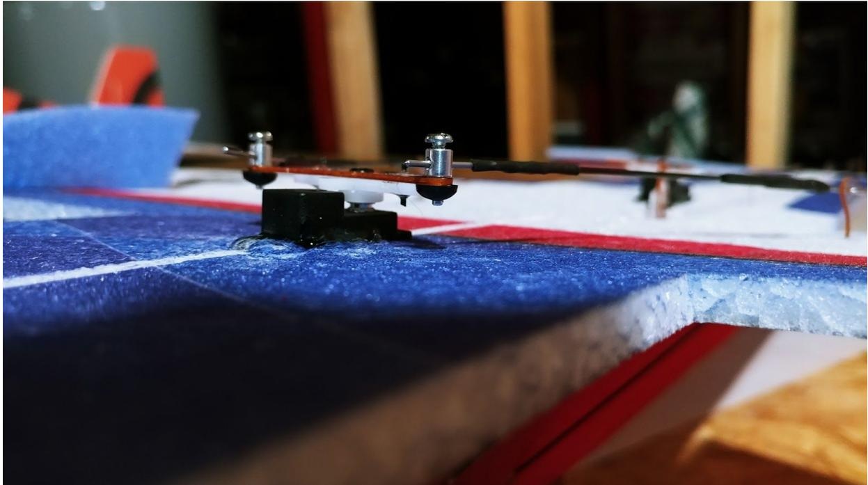
**Above is another photo showing the use of the mini EZ connector. These will be used to clamp the linkage to the rudder and elevator servo arms as well.**
