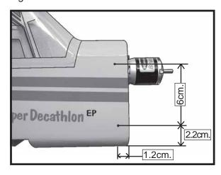
☐ 2) Slide the fiberglass cowl over the engine and line up the back edge of the cowl with the marks you made on the fuselage then trim and cut.
