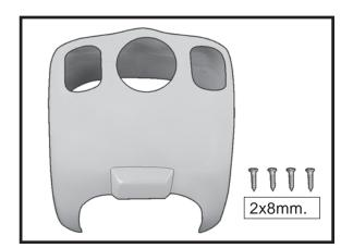
☐ 3) While keeping the back edge of the cowl flush with the marks, align the front of the cowl with the crankshaft of the motor. The front of the cowl should be positioned so the crankshaft is in **nearly** the middle of the cowl opening. Use the spinner backplate as a guide. Hold the cowl firmly in place using pieces of masking tape.
