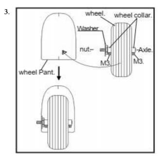
Place the wheel assembly in the wheel pants. The threaded portion of the axle will fit the notch of the wheel pant as shown.
