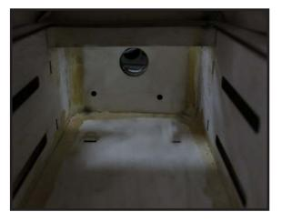
Drill a hole for the throttle pushrod.
