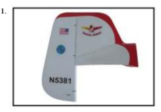
Using a modeling knife, remove the covering from over the precut hinge slot cut into the lower rear portion of the fuselage.
