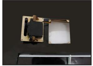
Set the aileron hatch in place and use a Phillips screw driver to install it with four wood screws.
