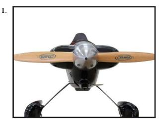
The propeller should not touch any part of the spinner cone. If it does, use a sharp modeling knife and carefully trim away the spinner cone where the propeller comes in contact with it.
