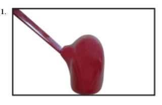
Repeat steps as above to attach remaining wheel pants to the landing gear.
