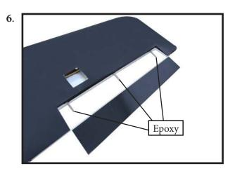
Be sure to test the aileron hinges once you insert them. Ensure that the hinge pockets line up, and that the hinges move freely before the epoxy dries.
