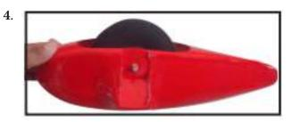
Slide the threaded end of the axle through the hole in the bottom of the landing gear leg. Use a washer and locknut to tighten the axle to the landing gear. Make sure to use threadlock on the nut so it won't vibrate loose in flight as shown.
