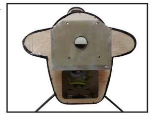
Use a 1/4 bit to drill the engine mounting holes. Remove mounting template from fie wall. Firewall shown with mounting holes drilled ready for engine mounting.
