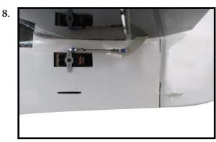
Thread one clevis and M3 lock nut on to each rudder and elevator control rod. Thread the horns on until they are flush with the ends of the control rods.
