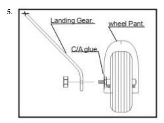
Tighten the setcrews using a hex wrench to secure the collars on the axle over the flat spot to retain the wheel as shown.
