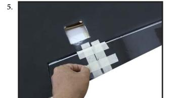
Because the size of servos differ, you may need to adjust the size of the precut opening in the mount. The notch in the sides of the mount allow the servo lead to pass through.
