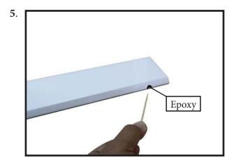
Apply epoxy into each of the holes in the ailerons using a spare piece of pushrod wire or toothpick.
