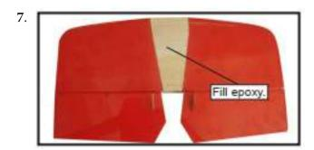
When you are sure that everything is aligned correctly, mix up a generous amount of 30 Minute Epoxy. Apply a thin layer to the top and bottom of the stabilizer mounting area and to the stabilizer mounting platform sides in the fuselage. Slide the stabilizer in place and realign. Double check all of your measurements once more before the epoxy cures. Hold the stabilizer in place with T-pins or masking tape and remove any excess epoxy using a paper towel and rubbing alcohol.
