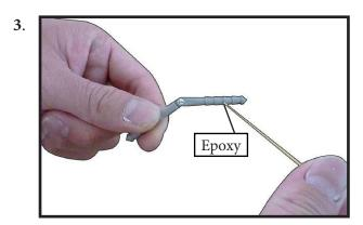
Apply epoxy to each hinge where it will be inserted into the ailerons. Tip: Apply some petroleum jelly to the metal pin hinge area to keep epoxy from interfering with smooth operation of hinge.
