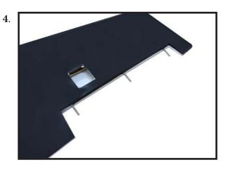
Insert all four hinges in the ailerons at this time. Make sure hinges move up and down in right direction and not side to side!
