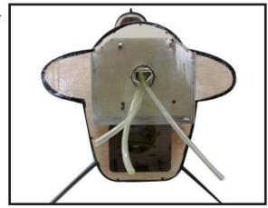
Connect the lines from the tank to the en gine and muffler. e vent line will connect to the muffler and the line from the clunk to the carburetor.
