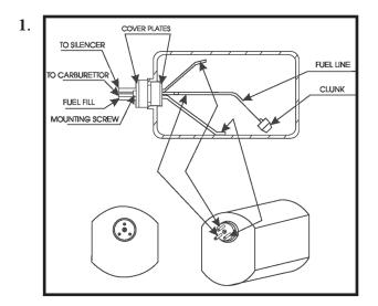
With the stopper assembly in place, the weighted pick-up should rest away from the rear of the tank and move freely inside the tank. The top of the vent tube should rest just below the top of the tank. It should not touch the top of the tank.
