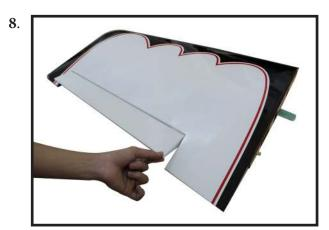
Check the fit of the aileron to the wing. The top of the ailerons will align to the top of the wing. Make sure movement is smooth and bind free.
