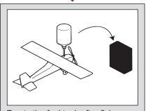
Empty the fuel tank after flying, the tank can corrosion and lead to problems.
