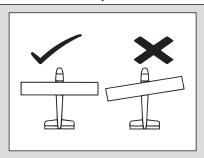
Check that the wings correctly fitted to the fuselage.
