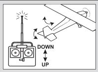
Operate the control sticks on the transmitter and check that the control surfaces move freely and in the CORRECT directions.
