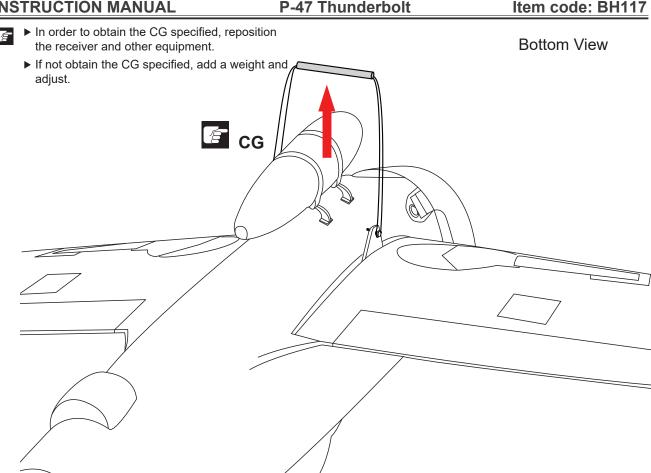
▶ Do not fly before confirming the correct location of the CG. If the CG is incorrect, you lose control of your airplane which leads to accidents.
