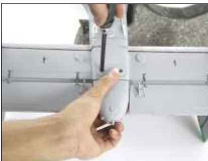
Connect the rudder servo cabin and Y-wire in fuselage.
