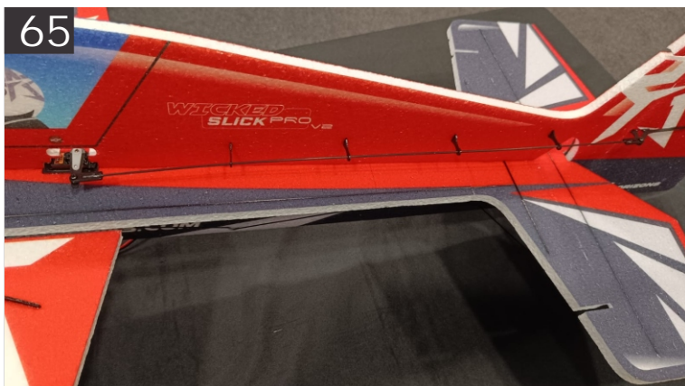
65. Above is the finished linkage setup with rudder centered and rod well fitted and glued in both the quick links with all the guides in place. Use the same process like we did in previous linkage setups.
