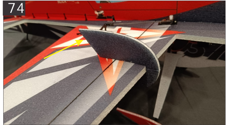
74. Slid in and glue the upper half of SFG using HV CA to the precut slots like shown in the above image.
