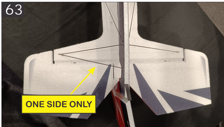
63. Install the last remaining 150mm rod to the bottom of the fuselage shown in the above image, this will be mounted from the bottom of the horizontal tail to the rear of the bottom vertical fuselage, make sure of full elevator deflection while installing this.
