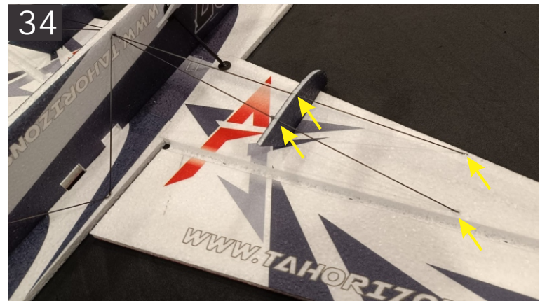
34. Glue the 330mm L X 4 rods for wing bracing. Make a small slot on bracing support using a sharp knife where it meets the rod, Make sure the carbon bracing is slid about a mm down into the slots. Glue it using a HV CA.
