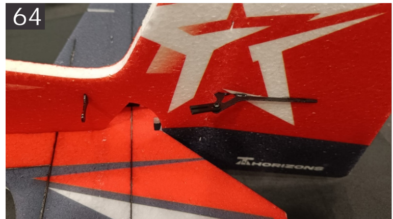
64. Install the last remaining control horn in the precut slot like we did for elevator horn. (Install it the opposite side of elevator horn)
