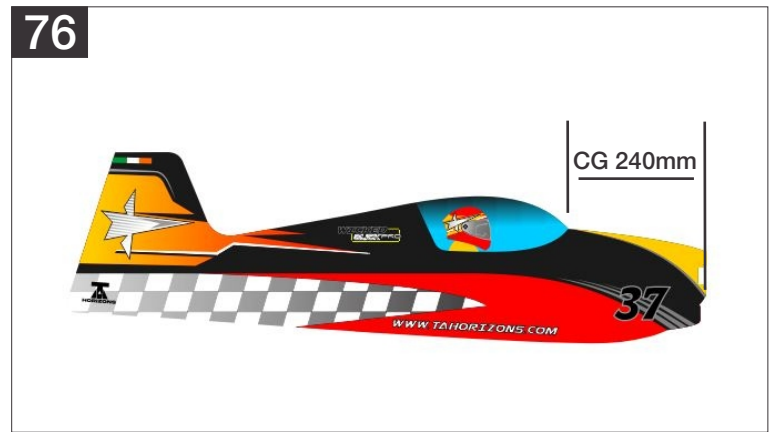
76. Initial CG is located 240mm from the nose of the aircraft (Not from the motor)
