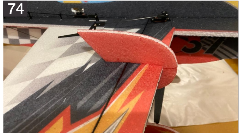
74. Slide in and glue the upper half of SFG using HV CA to the precut slots like shown in the above image.
