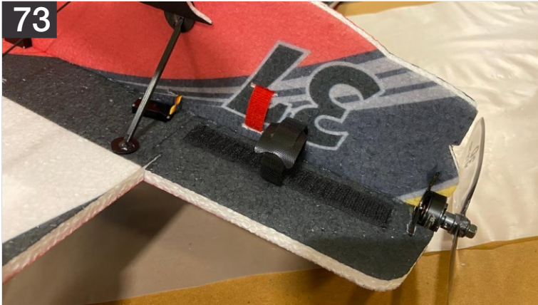
73. The long piece of velcro along with the strapping velcro mounted, above is the location of the battery for this setup.
