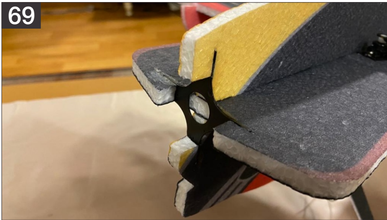
69. Shown above is the motor mount glued, making sure everything is flush and lined up correctly. After that install the motor on it.
