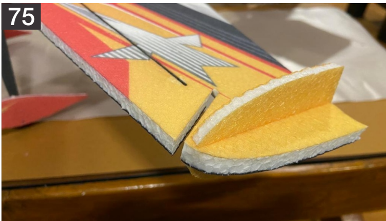
75. If desired, locate these smaller side force generators that will be glued into the counterbalances of the ailerons.
