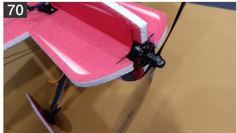
70. Enlarge the pre cut holes over the mount according to need and install the motor on it.
