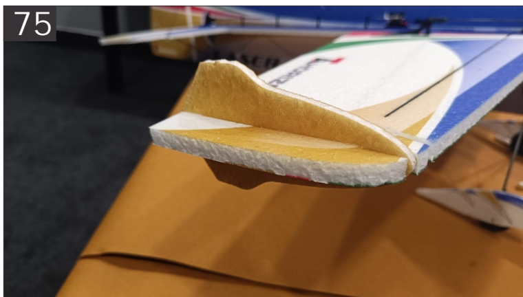
75. Here is how the side force generators are slid in and glued in the precut slots over the counterbalances of the ailerons.
