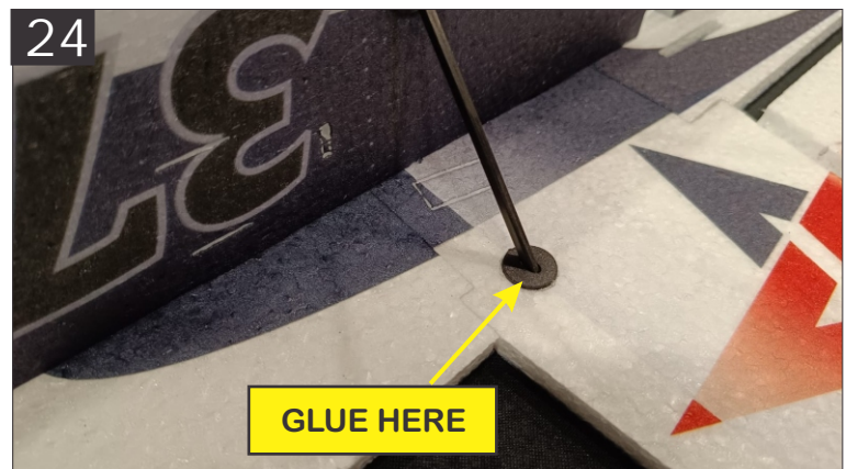
24. Put a drop of HV CA over the joints and spray everything together
