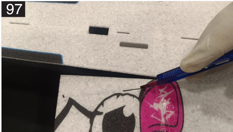
97. You will be required to widen down the aileron horn slot next to longer carbon rod slot, shown in the above image.
