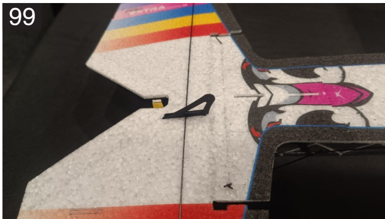
99. Glue the elevator horn shown in the image in the pre cut control horn slot using HV CA. Make sure it sits right to the bottom of EPP Surface.
