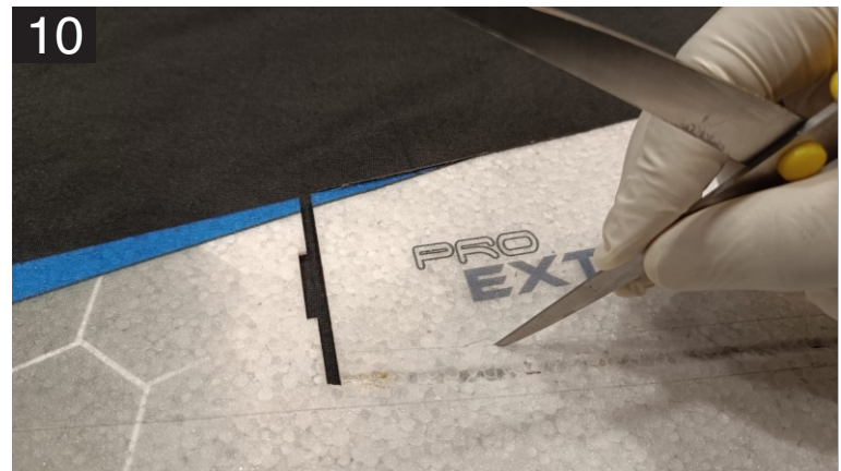
10. Turn back the wing to glue down the reinforcement rods, if needed use a scissor or a ball point pen to loosen down the pre cut laser groove lines.
