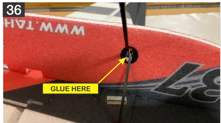
36. Put a drop of HV CA over the joints and spray everything together.
