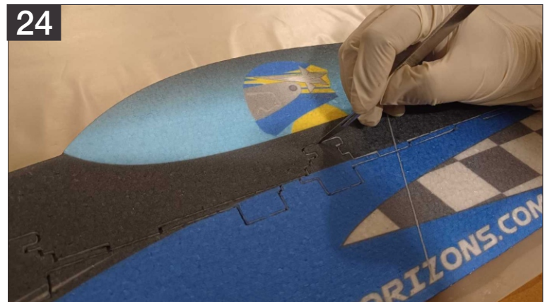
24. We can now began the vertical fuselage installation, use the blade to separate both the parts.
