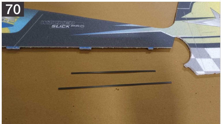
70. Before glueing the upper half of the fuselage, locate the 0.5X3mm (150mmL) stripe and 0.5X3mm (200mmL) stripe. these will be used to strengthen the vertical tail and rudder section.
