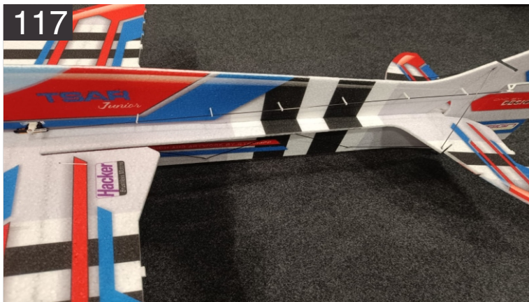
117. Above is the finished linkage setup with rudder centered and rod well fitted and glued in both the quick links with all the guides in place. Use the same process like we did in previous linkage setups
