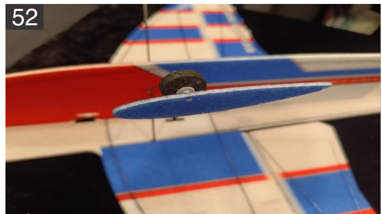
52. Glue the wheel pants on wheel stopper using the HV CA.
