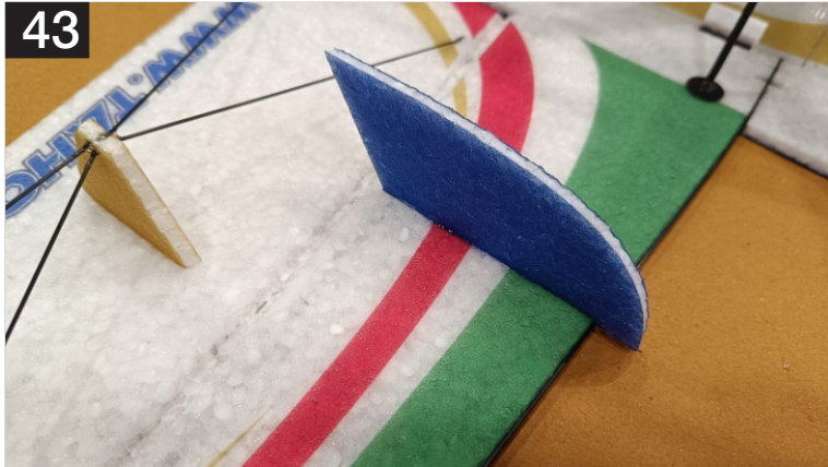
43. Locate and glue the half part of SFG works as wing truss support, glue it in pre-cut slot like shown in the picture.
