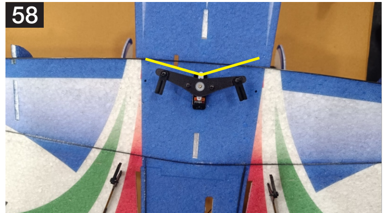
58. With the servo centered, Install the dual servo arm over it, check the orientation shown in the above image.
