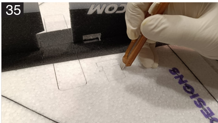
35. Take out the excess foam from the wing servo slots using the sharp knife.
