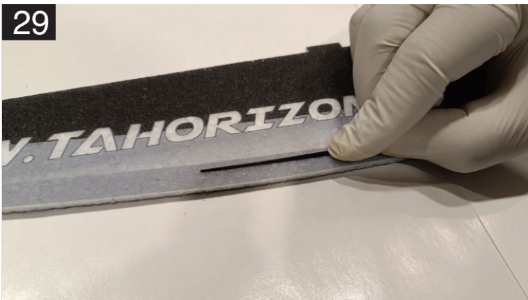
29. Belly of vertical fuselage also uses the 3 X 0.5mm stripe for reinforcement, Lay into it's designated slot, cut length as advised in the next step.
