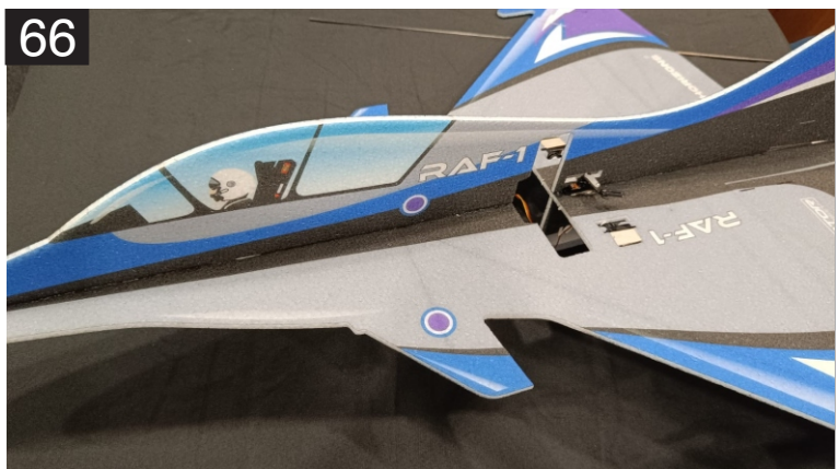
66. Engage all the tab and slots. Press firmly along the length of the fuselage to make sure all areas are fully seated. Check that the top piece is square and straight. Tweak if necessary to make it true.
