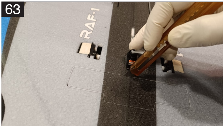
63. Cut out the excess foam for the motor mount using the sharp knife.
