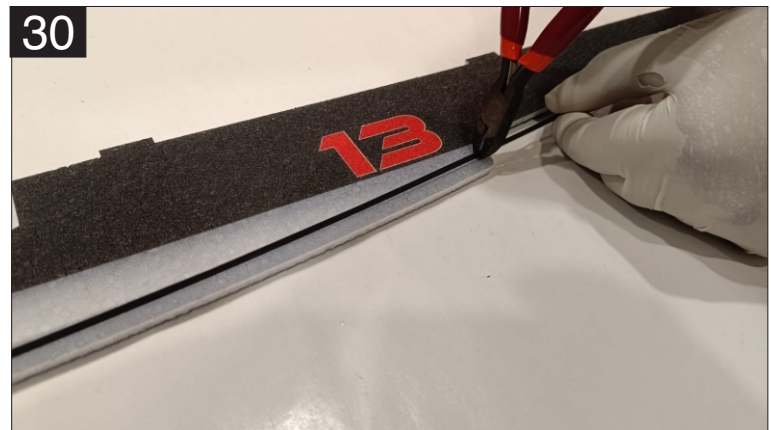
30. Once it reached at the end of Pre-cut slot, use a scissor or wire cutter to cut down the excess stripe.
