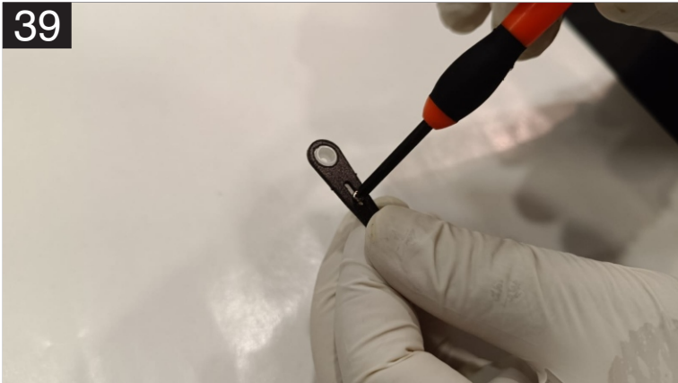
39. Install the extenders over the stock plastic servo arms using the small screw. Wrap with thread for more strength if desired.
