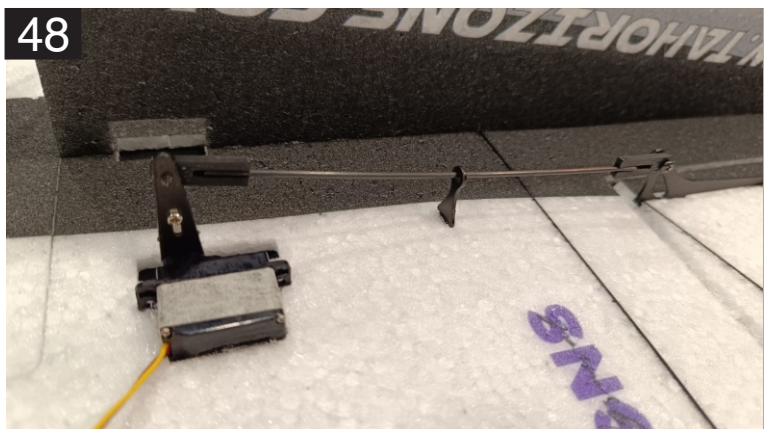
48. With the servo arm and control surface centered, dry fit the control rod as shown above.
