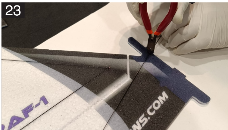
23. Use a scissor or wire cutter to cut down the excess stripe.
