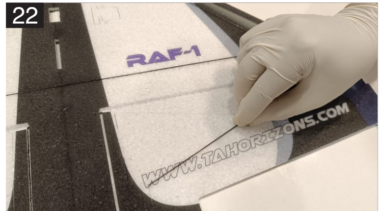
22. Use the same 3 X 0.5mm stripe to reinforce the elevons as well. Glue one of the two carbon stripes that goes in cross shape in the elevons as shown above.
