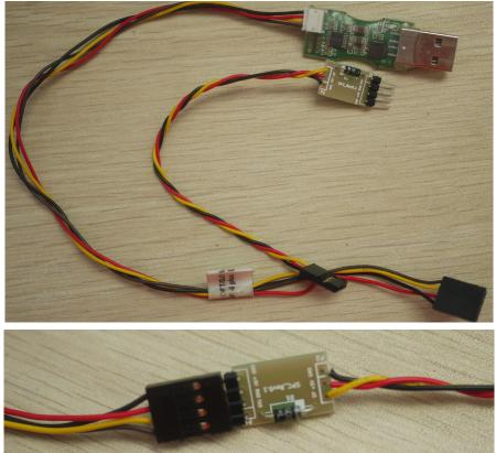
Step 2: Change pin sequence, and remove the 5V pin.
