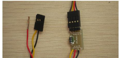
**Step 3:** Plug the "Ground" and "Smart.Port" pin to the back of the Taranis like this.
