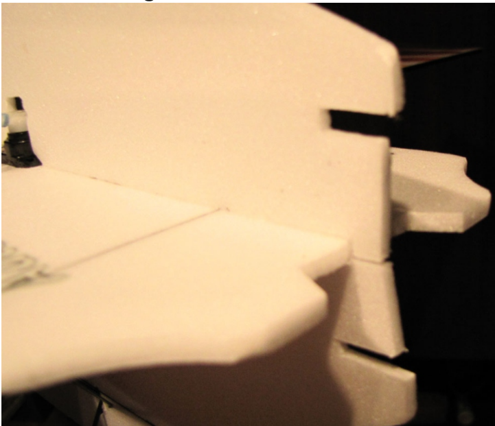
Depron cut out for motor with TVR system.
