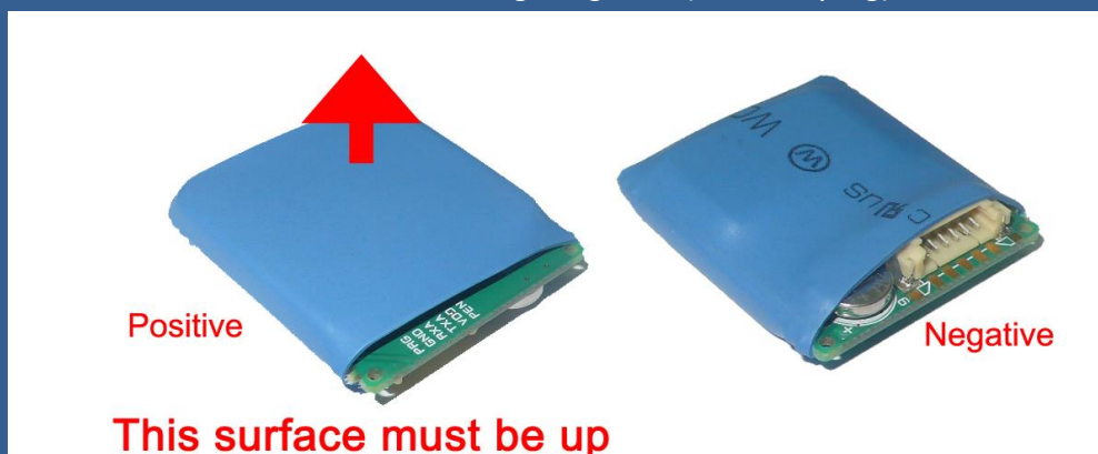
GPS Module Installation
